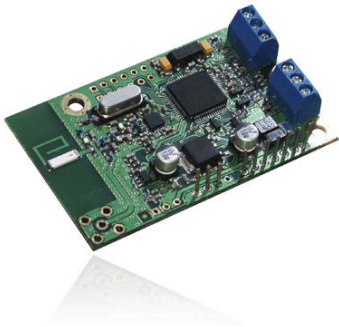
EW1 - wireless zone and PGM output expansion module
