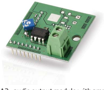
EA2 - audio output module with amplifier
