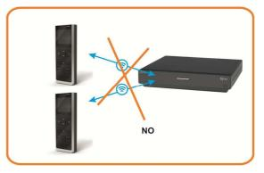
To link a Remote with a Main Speaker or Zone Controller, press the "link" key □ and select the Main Speaker or Zone Controller from the list that appears on the screen.
