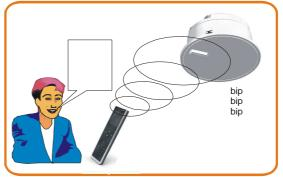
This mode is active while the person continues to speak (maximum time: 1 minute). The autoresponse sensitivity and silence time are programmable parameters (see section 5.3).
