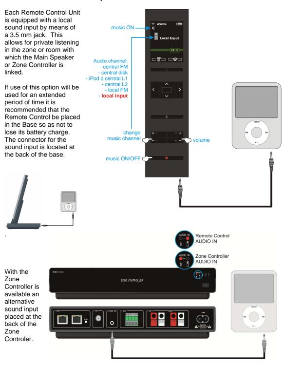
The Sound input at the back panel of the Zone Controller (AUDIO IN) is shared with the same input for the Remote Control, and can be actived one at a time with priority for the Zone Controller input. Only when there is any jack connected in the Zone Controller, the external sound source will be available for the Remote Control.
