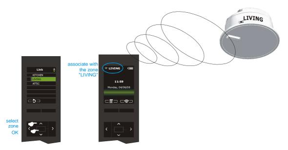
If the desired zone does not appear, it is outside the coverage area. Go closer to the Main Speaker or Zone Controller with which we want to link and select a zone (see section 1, recommendations for optimal communication between Remote Control and Main Speaker or Zone Controller).
