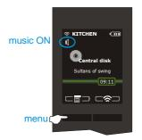
Select the audio levels menu for access to the levels of volume, balance, treble, bass, loudness activation/deactivation and activating the timer to turn off the music automatically in accordance with the time programmed.
