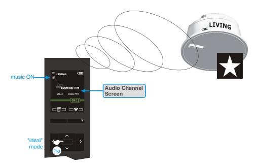
The available settings to be stored in "ideal" mode are levels of volume, balance, bass, treble, loudness, audio channel and FM tuner station (if the audio channel is an FM tuner). To save as "ideal" mode, proceed as follows:
