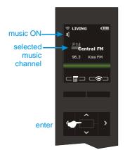
To navigate advanced settings and program memories on either tuner, press the central navigation key ("enter").
