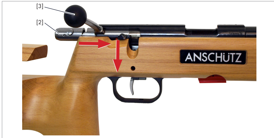
Fig.4 Closing the breech
