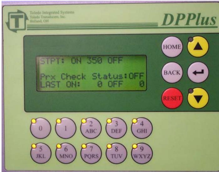
This input is used to check for encoder slippage. The prox should be mounted so it will cycle in the same spot every stroke. Set the STPT: ON/OFF so it will alarm if the encoder slips. These settings are set up the same way as a Die Protection station with static with window and N.O. Contact. (See Section 6). The STATUS and LAST ON/OFF are diagnostics to aid in setting the proper setpoints. To disable this input set both ON and OFF to Zero.
