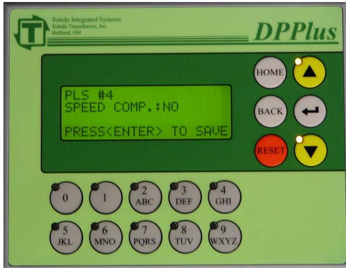
The above screen will appear to allow the Speed Compensation to be set on or off for the PLS. If Speed Compensation is required, select “Yes”, otherwise select “No”. Use the up and down arrows to change the setting. When the correct value is displayed, press the <ENTER> key to save the changes. For an explanation of Speed Compensation, refer to Section 8.2 Speed Comp PLS.
