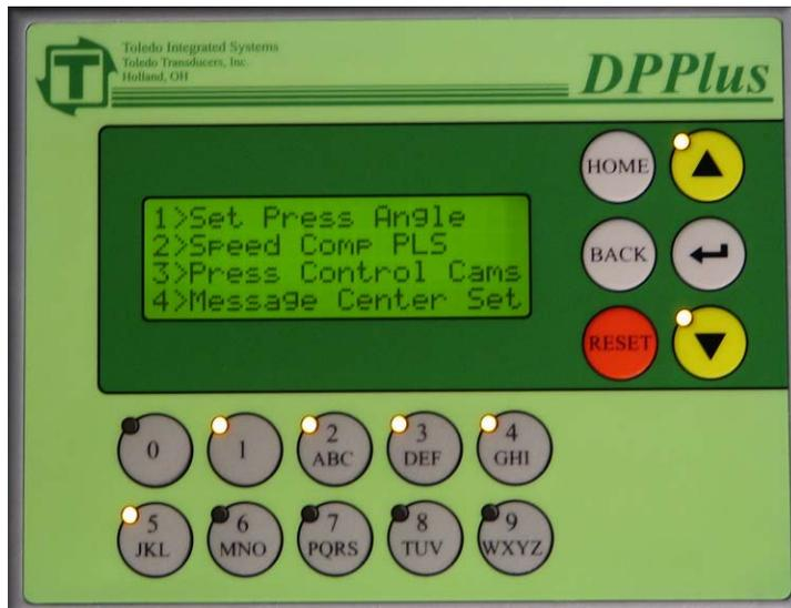
After the correct password has been entered, the Calibration Menu screen (shown above) will be displayed. The following 5 options will be listed: Set Press Angle, Speed Compensation PLS, Press Control Cams, Message Center Setup, and Restore Defaults. Use either the alpha-numeric keys or the arrow keys to select which Calibration Procedure to perform. When the correct selection is flashing, press the <ENTER> key.
