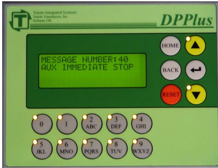
The screen will display the Message to be modified; the new message text will be entered below the current message. Use the alpha-numeric keys to enter the new Message. For instructions on entering text, refer to Section 11 Text Entry. When the new Message text is entered correctly, press the <ENTER> key to apply the changes. Press the <BACK> key to return to the previous screen to select more Messages to modify.
