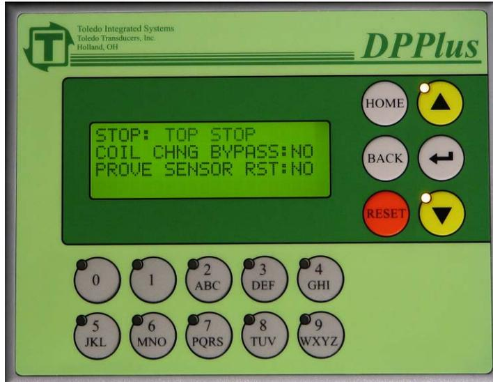
Pressing the <BACK> key will display these additional settings. Press the <BACK> key again to return to the Die Protection Selection Menu.
