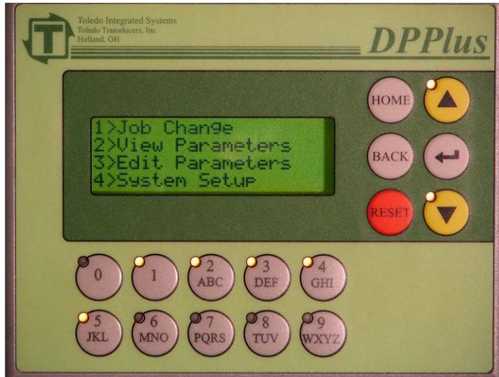
From the Menu Select Screen, you can maneuver to the different settings within the DPPlus. The following five functions can be accessed from this screen: Job Change, View Parameters, Edit Parameters, System Setup, and DPPlus Calibration. To protect the system settings, a password is required for all functions except View Parameters.
