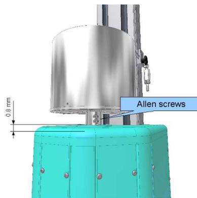
Figure 16: Mounting the outer vessel of the Viskomat XL.
