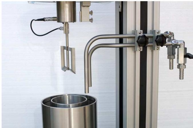
Figure 10: Tubes in the maintenance position, you may now remove the double wall container.
