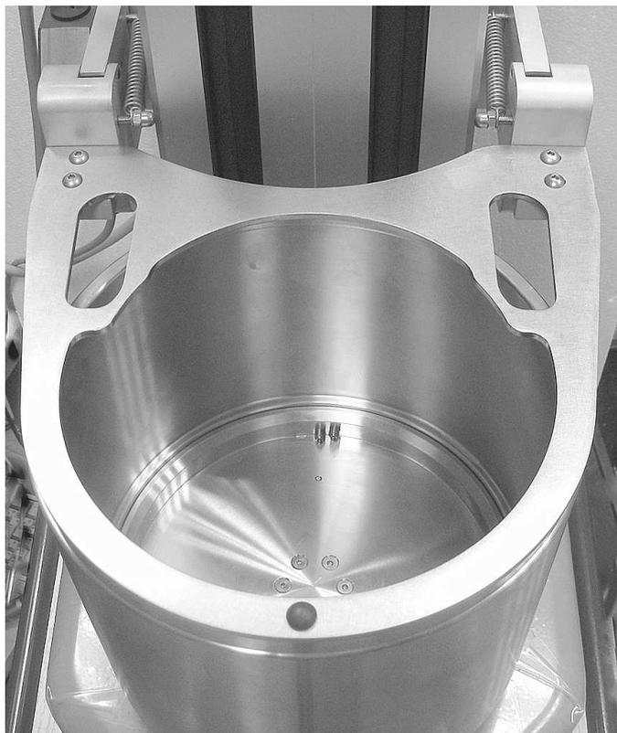
Figure 11: The safety guard of the viskomat XL in the working / normal position
