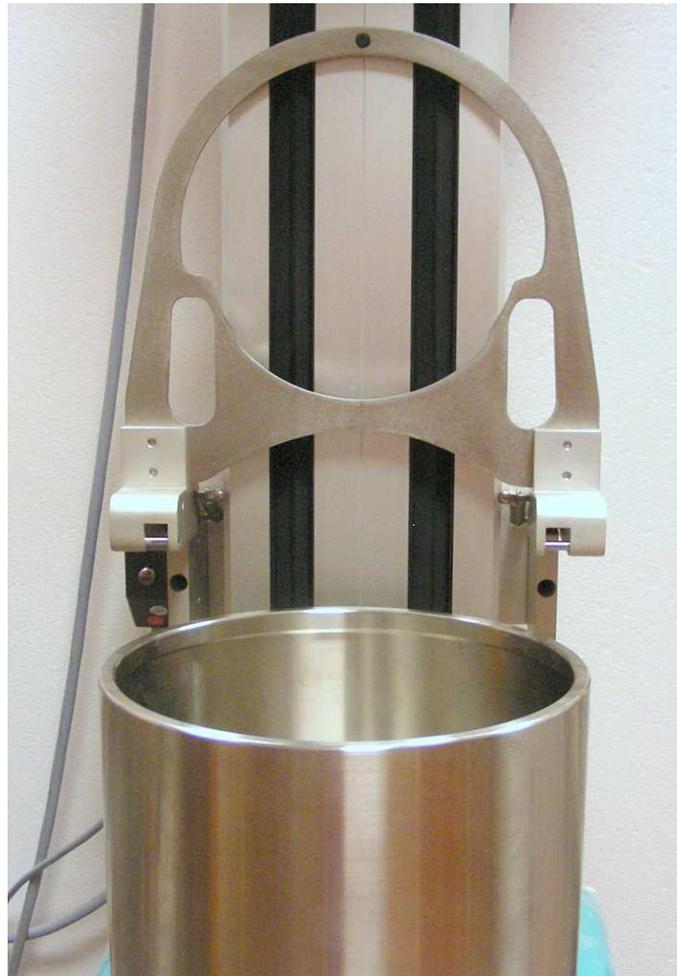
Figure 12: The safety guard of the viskomat XL in the opened position
