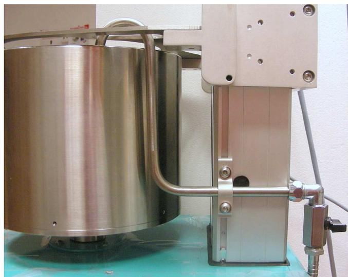
Figure 13: The tubes of the viskomat XL in normal operating position
