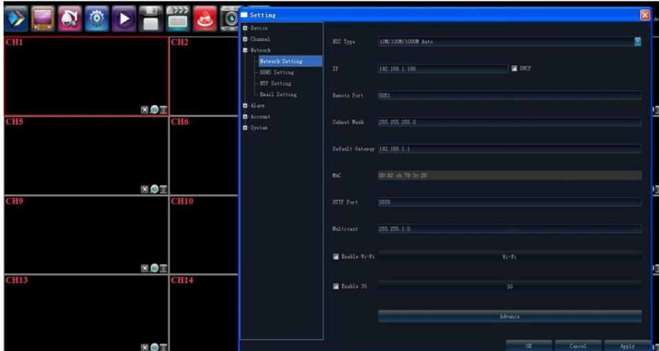
3. We need to map the ports of the NVR in the router, the ports are **HTTP Port:5555**、**Remote Port:5051** and **Mobile Port:5054 (Mobile Port =Remote Port + 3)**.
