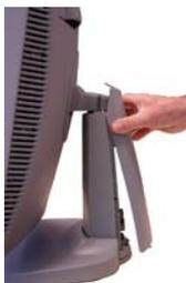
Push the upper side of the cover onto the foot
