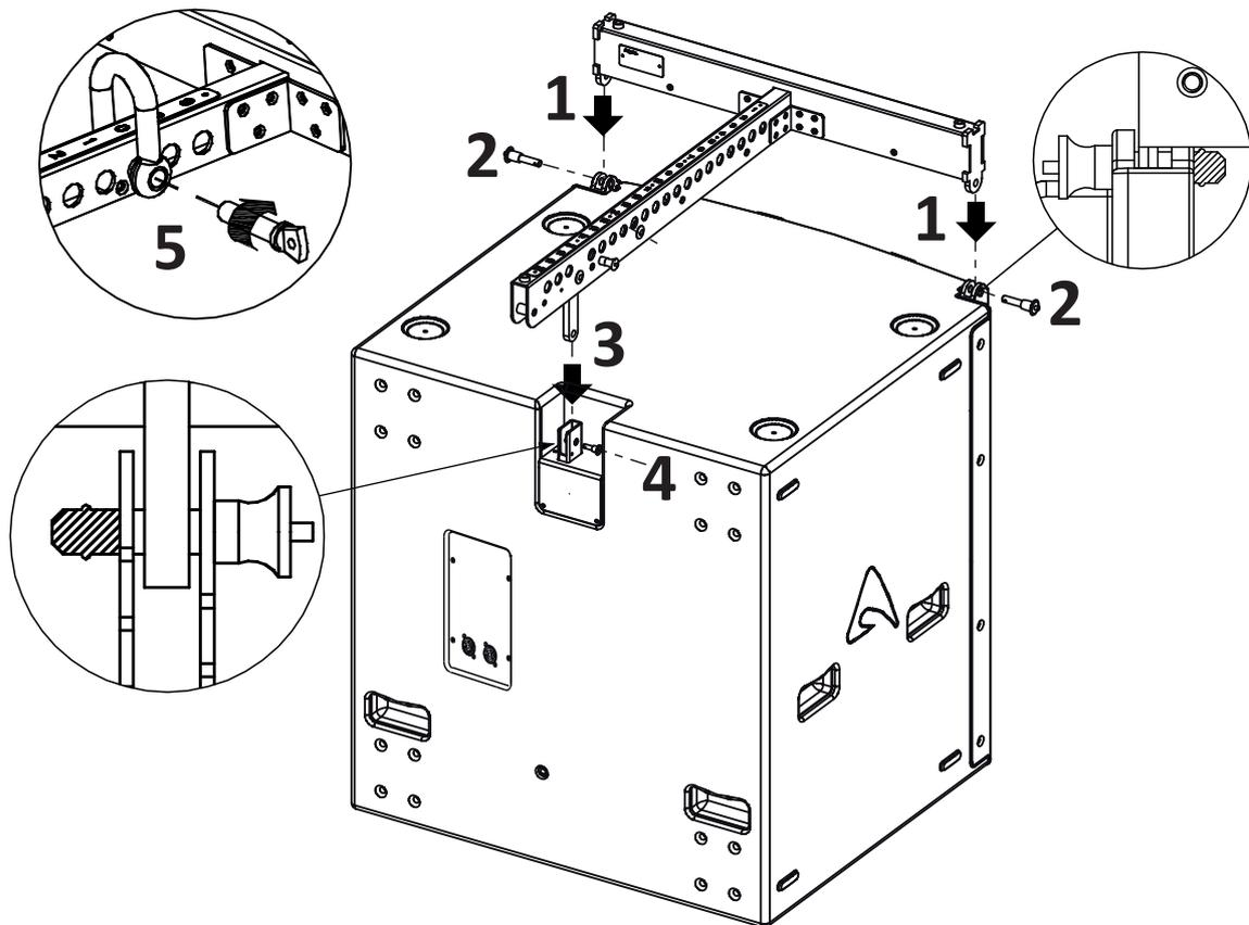
Follow the sequence in the figure for fixing the fly bar at the first box. Usually this is the first step before lifting up the system. Be careful to insert properly all the locking pins (1)(2) and (3)(4) then the shackle (5) in the right holes as specified by the aiming software.
