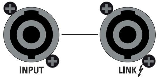
**LINK** - Power output in parallel with the INPUT socket for connecting the unit to another speaker. The number of SW215P cabinets that can be connected in parallel depends on the amplifier load capacity.
