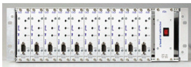
Installation in a base unit with 10 modules and common power supply.
