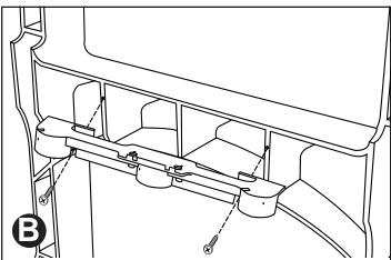
Assemble the Upper Bracket onto the back of the top step using two of the screws supplied.
