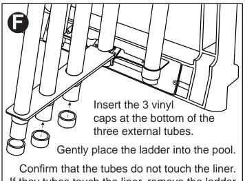
If they tubes touch the liner, remove the ladder from the pool and cut the tubes.
