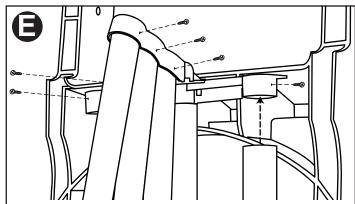
Insert 3 barrier tubes through the Lower Bracket and secure with one screw on each tube to the Upper Bracket.
