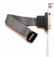
8-bit I/O extension on a slot plate
