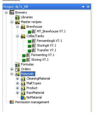
In the Fermenting- and Storage cellar a batch is started for every vessel. In the present example only the technological Steps for filling or emptying respectively are implemented. This Steps are located in the following recipes:
