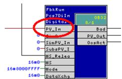
The input or output signal are defined as textual interconnection in the CFC chart.
