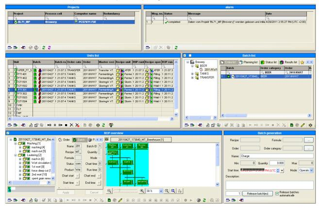
The process picture "Batch-Controlling" contains sub-windows for the following Batch OS-Controls (See SIMATIC BATCH Manual Chapter BATCH OS Controls for further details ):
