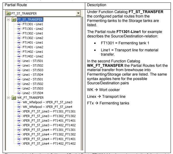
The associated function definitions of Partial Route **FT1301-Line1** are shown in the following picture. The Control-, Sensor-, Parameter- and Link-elements are assigned to the partial route and the control function is selected and checked:
