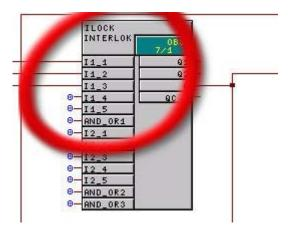
Three interlocks are connected to textual interconnections, the other interlocks are unused. Interlocks are engineered after import of the modules by using the symbolic names of the I/O signals.
