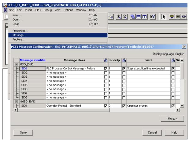
In message section you define message class, priority, message text as an event and acknowledge action. Message class should be alarm, warning, tolerance and etc. In the Event field you can type the message text.
