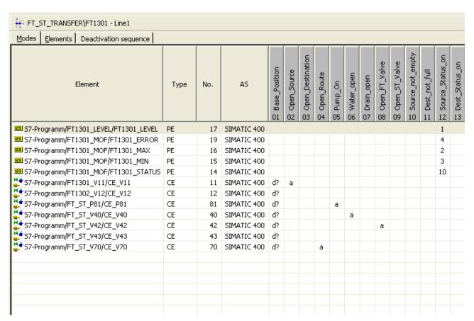
As an example - the state of tank valve FT1301\_V11/CE\_V11 is checked passive (d?) in function "01-Base\_Position" and is activated (a) in function "02-Open\_Source".
