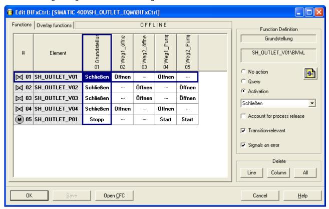
The possible routes are defined as functions of the BIFCtrl block. In the function definitions (columns) the commands of the involved CMs (V01 – V04, P01) are configured. At runtime the function number is forced in the SFC OUTLET\_EX and the control and monitoring of the control modules is processed independently in the BIFxCtrl block.
