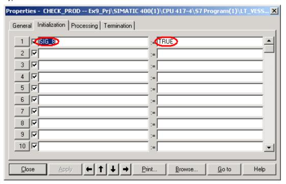
For reactivating the same alarm you have to reset the input signal. This should be located in the END step of SFC-Type.
