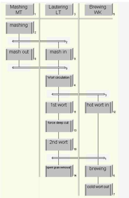
The activity of the recipe functions (RFs) to the according ROP is shown in the second recipe level. In the recipe functions the EQM-Phases (SFC-Types) with the control strategies and setpoints are called
