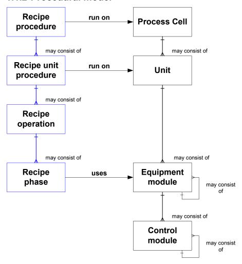
The control modules consists of blocks from the PCS 7 BRAUMAT Library and the PCS 7 Advanced Process Library (APL) and and prepared and tested for the use with two level recipes (Recipe operations and Recipe phases. The recipe phases corresponds with equipment modules implemented with SFC-Type). However the library blocks may be used basically also with single level recipes, where recipe operations corresponds with equipment operations which are implemented with SFC-Type.
