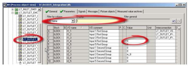
By selected the right chart within the plant hierarchy (Tree-view on the left) all signals which are labeled as 'parameter' are shown in one list. By using a suitable filter only the relevant signals for the interlocking are in one list.
