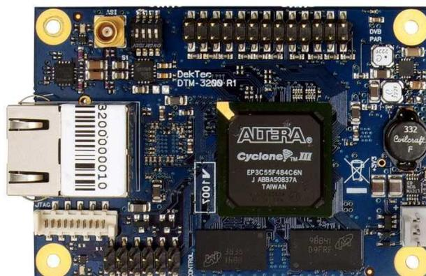
Figure 1. The PCB of the DTM-3200
