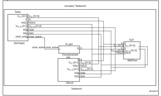
Figure 2. Testbench
