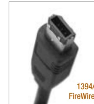
**Caution: Use only one interface at a time.** If you connect both the USB and the IEEE 1394a cables to the same external drive at the same time, you could damage the drive. However, it is OK to connect two IEEE 1394a/FireWire cables to the same drive at the same time to daisy-chain devices.
