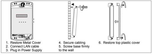
Check all sensor cables are securely tied down. Restore the metal cover to ensure safe installation. Plug in the DC jack and the LAN cable. Firmly screw down the Energy Monitor base to the wall and screw down the top plastic cover. The system is now ready to power up.
