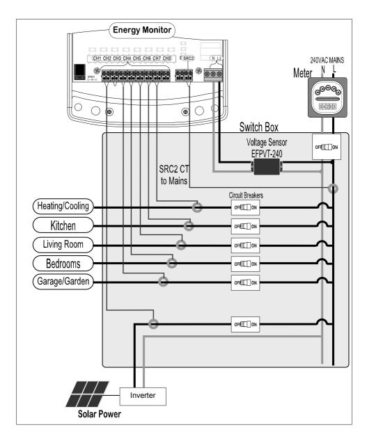
**Note:** For solar systems only CH1 can be used to measure the AC solar input circuits. This must be configured in software.
