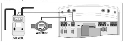
Note: Gas and water meters must have a pulsed output signal.
