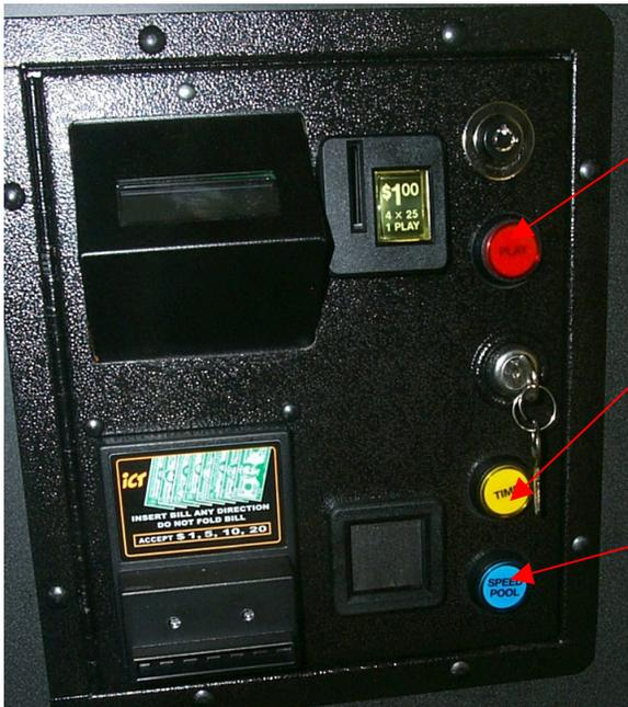
The PLAY button is used to go up through menu options, and when data is flashing, pressing this will increment that data.
