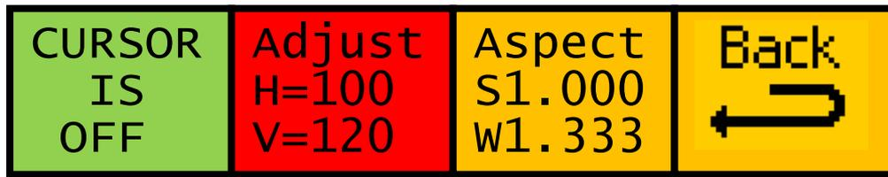
Pressing the first menu button or adjusting digi-pot 1 will toggle the cursor on and off. If another special purpose cursor is being displayed it will be removed. The width and height of the cursor can be adjusted by opening the “Adjust” menu and using digi-pot 1 and 2. The W and S values indicate the aspect ratio of the user box when viewed in standard aspect ratio (4:3) and widescreen aspect ratio (16:9). For HD signals only the W value is active.
