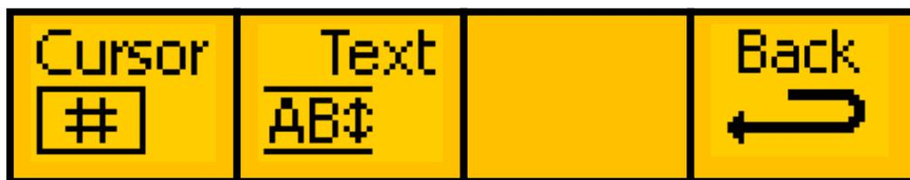
Pressing “Cursor” displays the menu detailed in section 3.3.6. Pressing the “Text ABC” menu displays the menu detailed in section 0. Pressing the “Back” menu takes you back to the top level menus.
