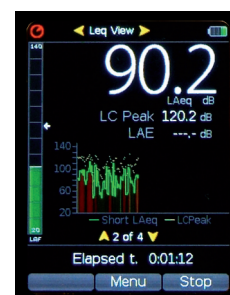
Leq screen with LAeq,t, Peak(C) and LAE
