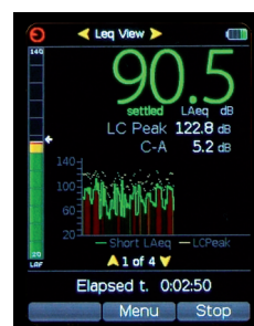
Leq screen with LAeq,t, Peak(C) & C-A values with the Leq value settled
