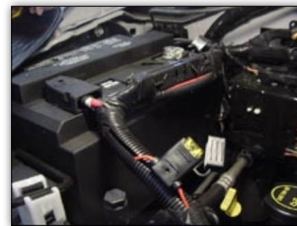
Main power connects at the battery with a fuseholder to protect the wire
