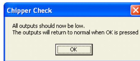
**Check timing:** The 'Check Timing' routine toggles the standby data line 200,000 times and puts a 10 KHz square wave on the data line for 10 seconds. The cursor should change from an arrow to an hourglass for approximately 10 seconds if the timing is correct.
