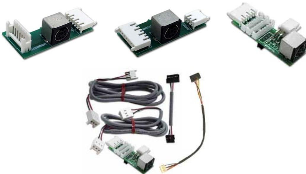
In addition to the TECI1 adapter and cables, there are replacements for the legacy adapters. These replacement cables connect to the TECI1 adapter and provide connection to older legacy sets.
