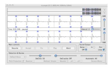
Looking at the figure, notice that "Default Brass" settings are in use – this employs "Pitch Protection". Every pulse has been identified as a potential click, which would lead to the destruction of the trumpet sound rather than the removal of noise. But they have also been identified as due to high-energy pitch, and no modifications made. This is indicated by the use of blue, rather than red, in the display and in the sound bar.
