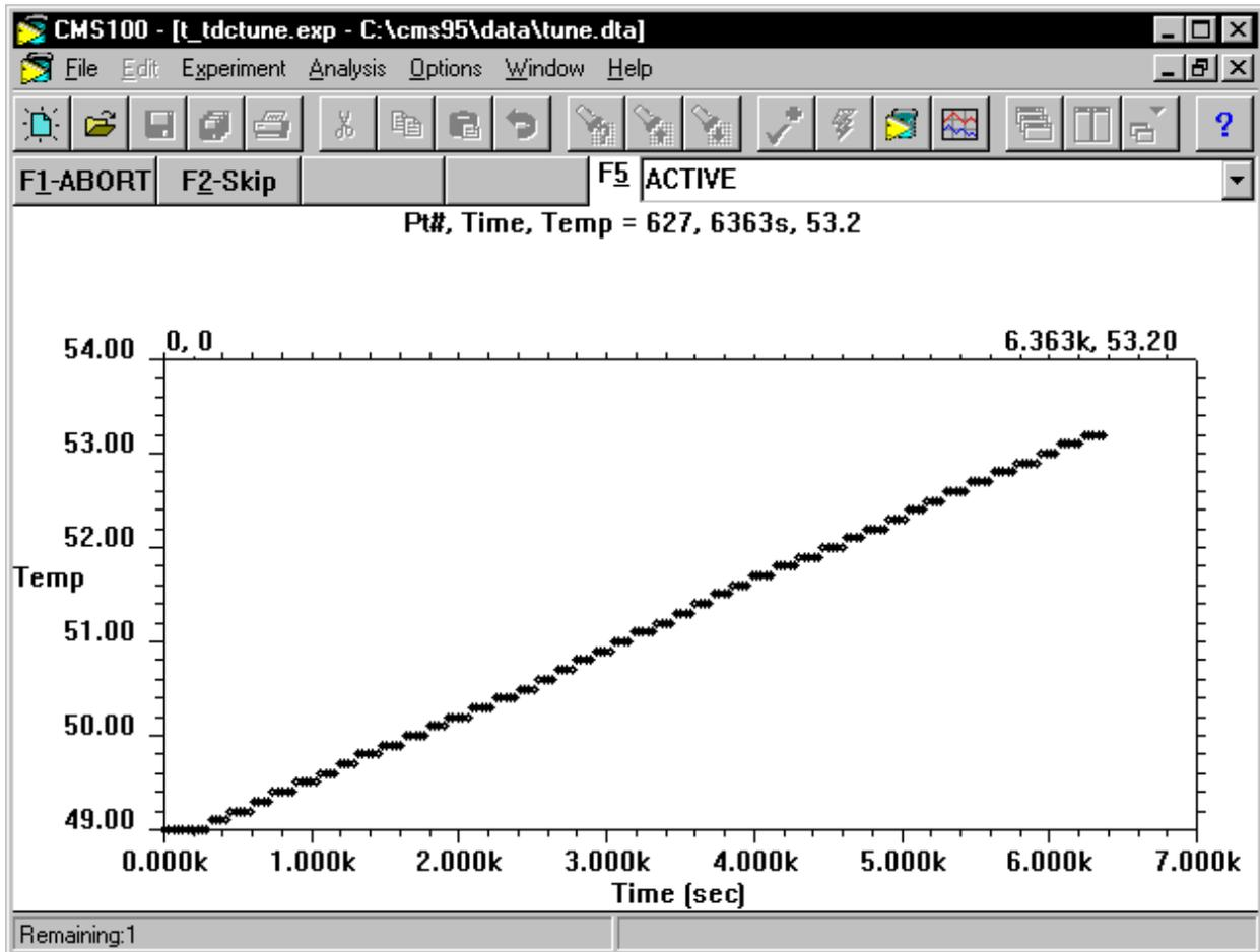
Wait until some curvature is seen in the temperature versus time curve. Figure 3-1 shows a good quality curve. Select F2-Skip to terminate the experiment.
