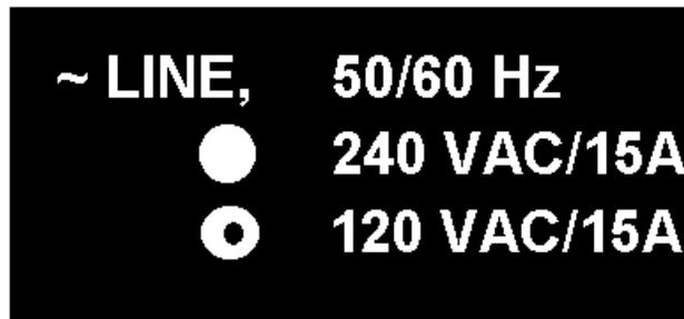
Before plugging in your TDC2 Temperature Controller you must check that its AC line voltage setting matches the voltage of your AC power line.
