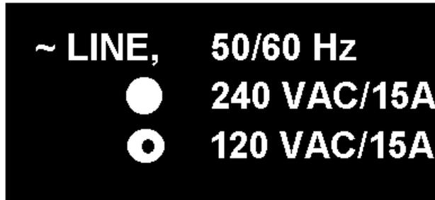
Check that the TDC2 has been wired for the voltage range appropriate for use in your area.
