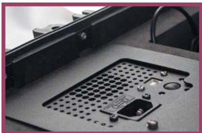
Figure 14 Weatherproof mains connection
