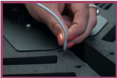
Figure 10 Routing leads to device slots
