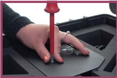
Figure 7 Unscrewing power unit
