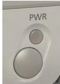
Figure 4-6 On/Off Button on Operator Panel
