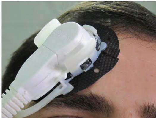
Figure 5-7 Sensor Connected to the Smart Pad
