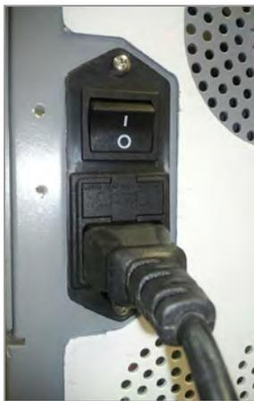
Figure 4-4 Connecting the AC Power Cable to the c-FLOW™ Monitor
