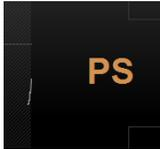
During Monitoring, in the event of any occurrence of poor Sensor signal strength, this will be shown in the display (for that corresponding parameter and Sensor) by the measured value indicator changing from a numeric value to **PS** (indicating poor signal). For suggested corrective action, refer to [Appendix A - Troubleshooting Guide](#)
