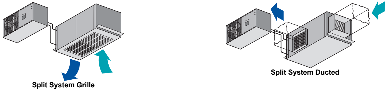
Figure 3 Split system air cooled systems
