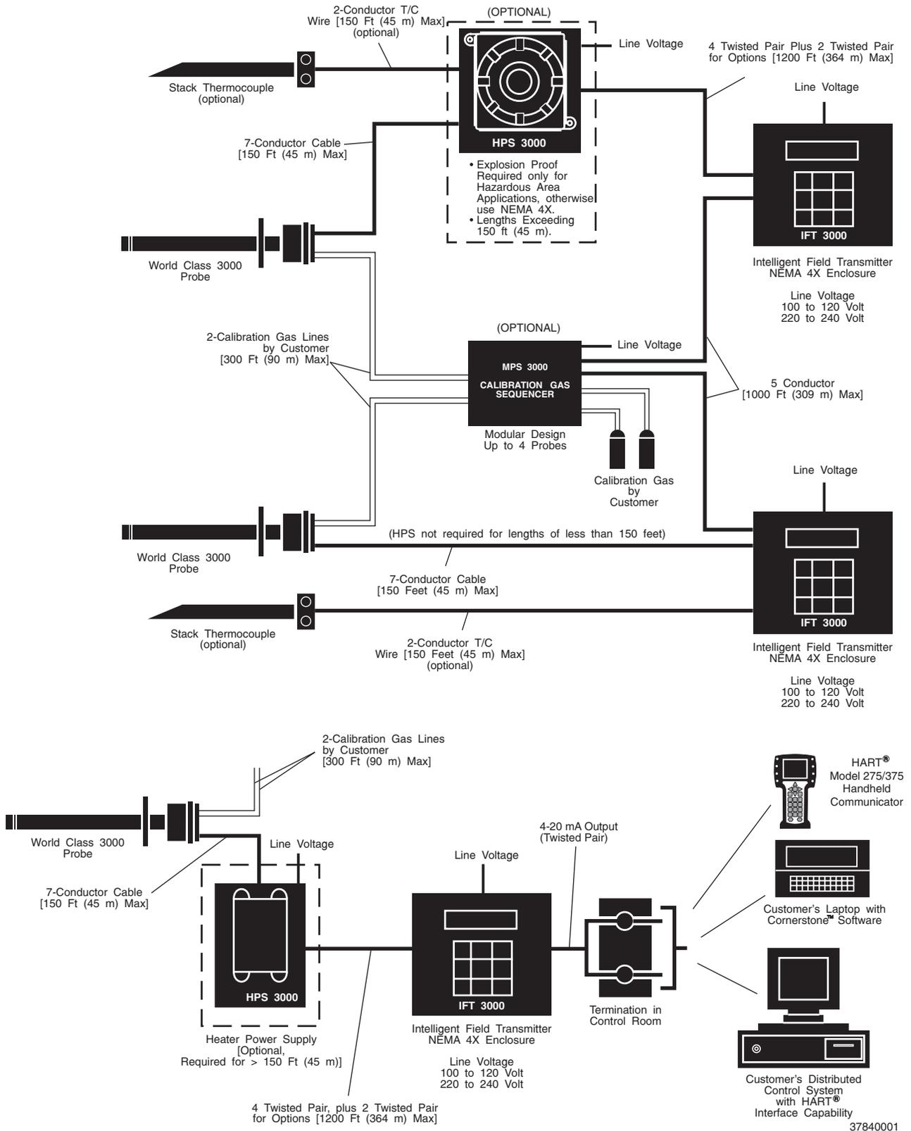
**Figure 1-3. World Class 3000 Typical Application with Intelligent Field Transmitters**
