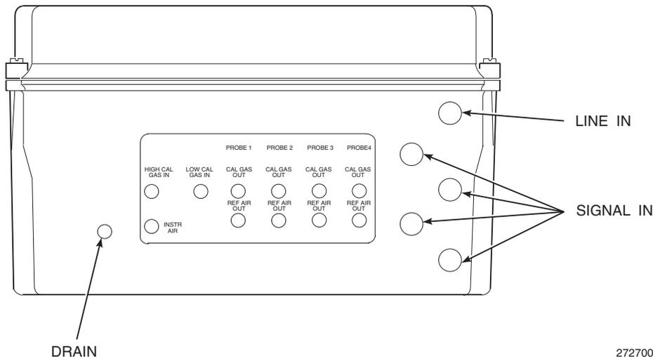
**Figure 2-18. MPS Gas Connections**
