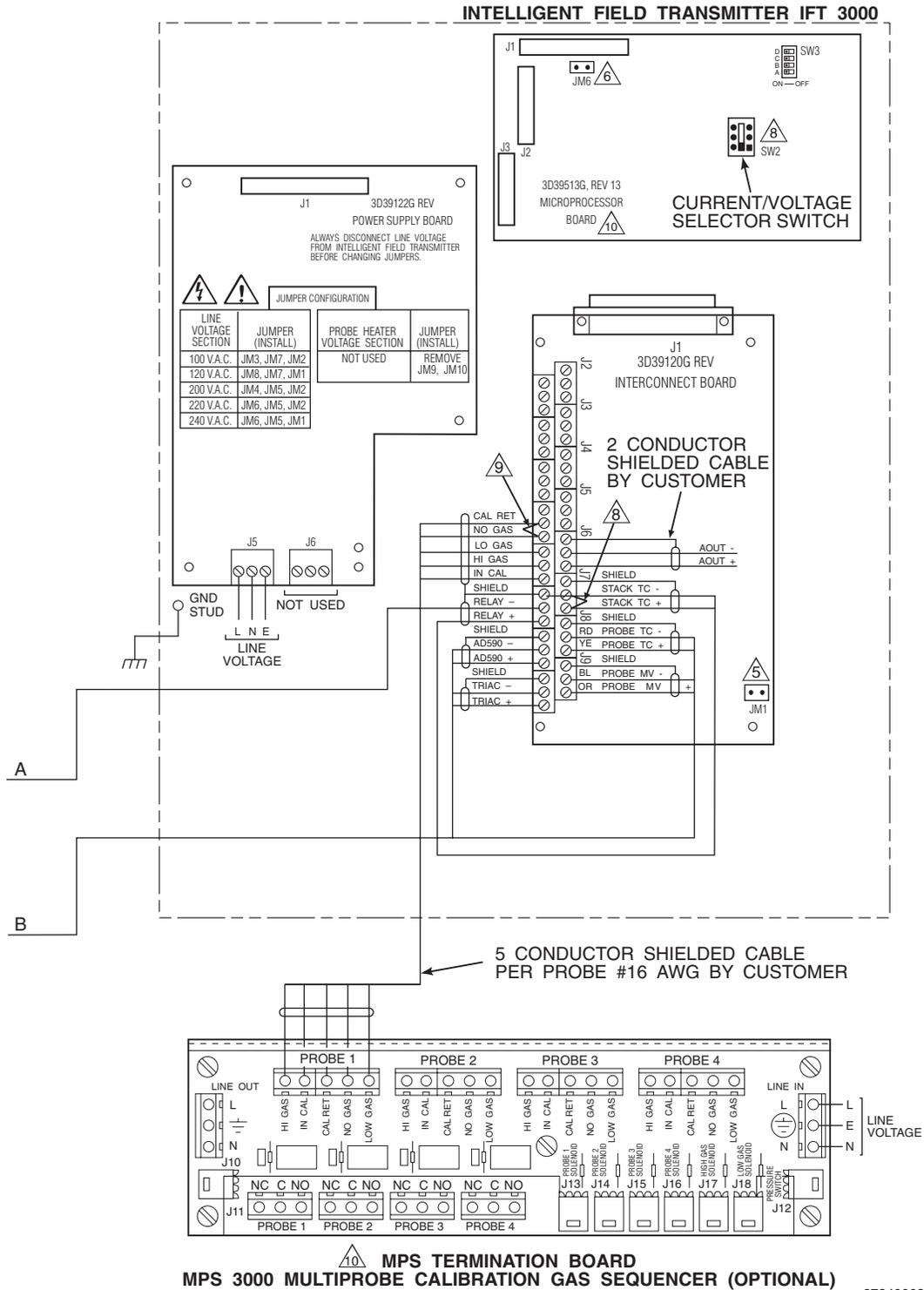
**Figure 2-13. Wiring Layout for Complete IFT 3000 System with HPS (Sheet 2 of 2)**
