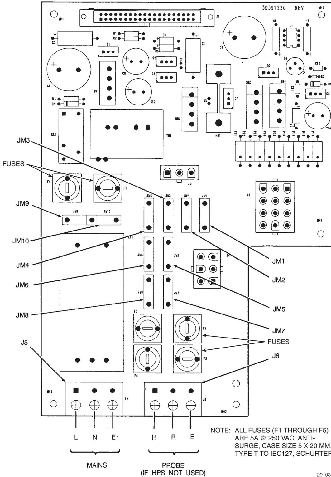
Figure 2-6. IFT Power Supply Board Jumpers
