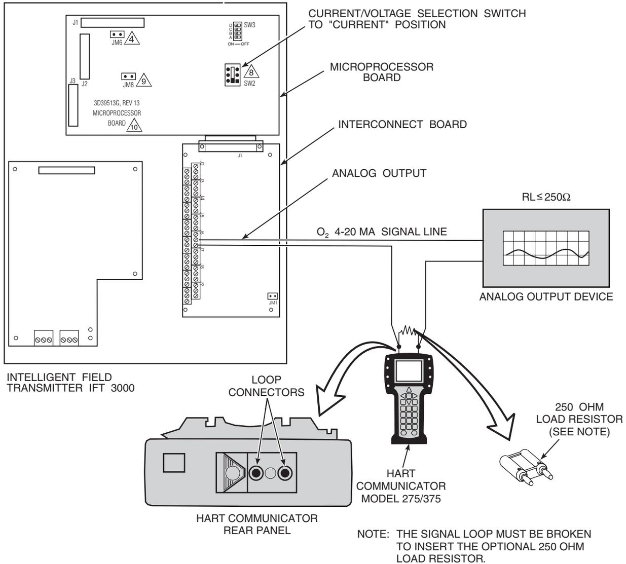
Figure J-3. Signal Line Connections, < 250 Ohms Load Resistance
