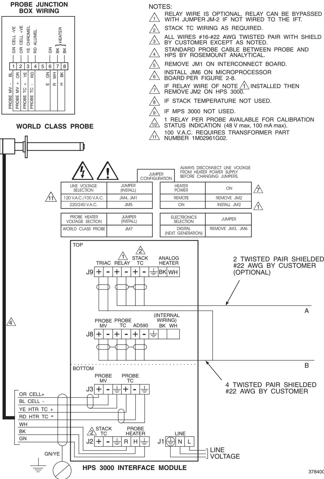
**Figure 2-13. Wiring Layout for Complete IFT 3000 System with HPS (Sheet 1 of 2)**
