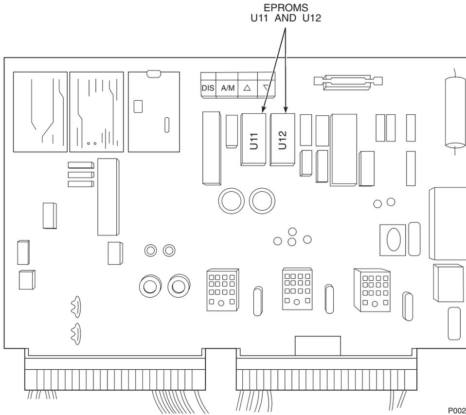
**Figure 2-11. Main PCB (Model TC200) EPROM Replacement**
