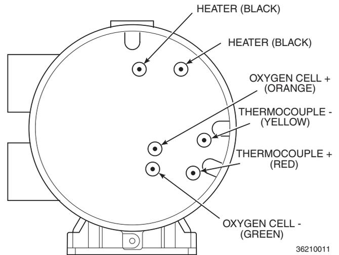
**Figure 4-6. Termination Housing Connections**
