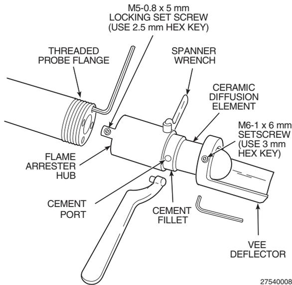
**Figure 4-5. Ceramic Diffusion Element Replacement**
