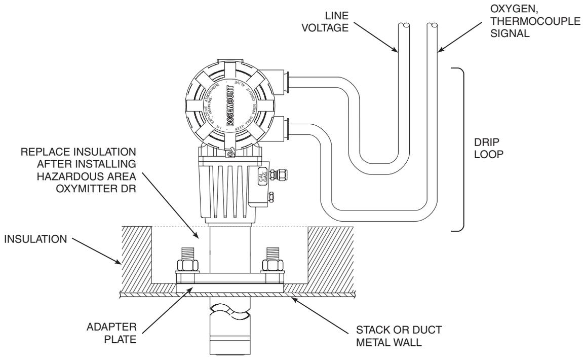
**Figure 2-6. Installation with Drip Loop and Insulation Removal**
