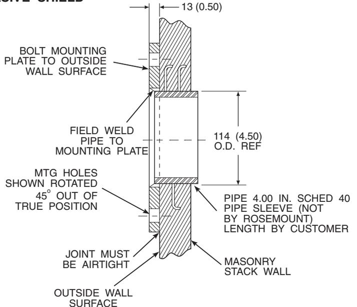
NOTE: ALL MASONRY STACK WORK AND JOINTS EXCEPT ADAPTOR PLATE NOT FURNISHED BY ROSEMOUNT.
