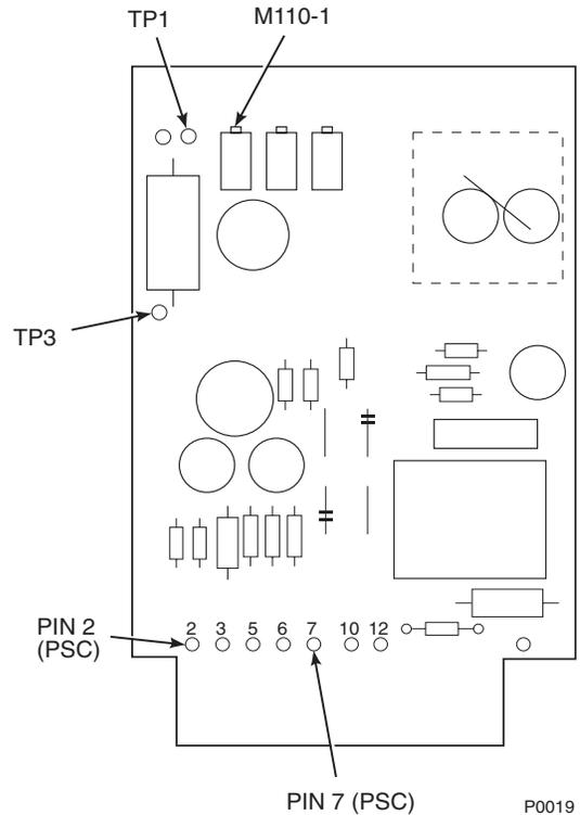
**Figure 2-9. Temperature Controller Card Calibration Points**
