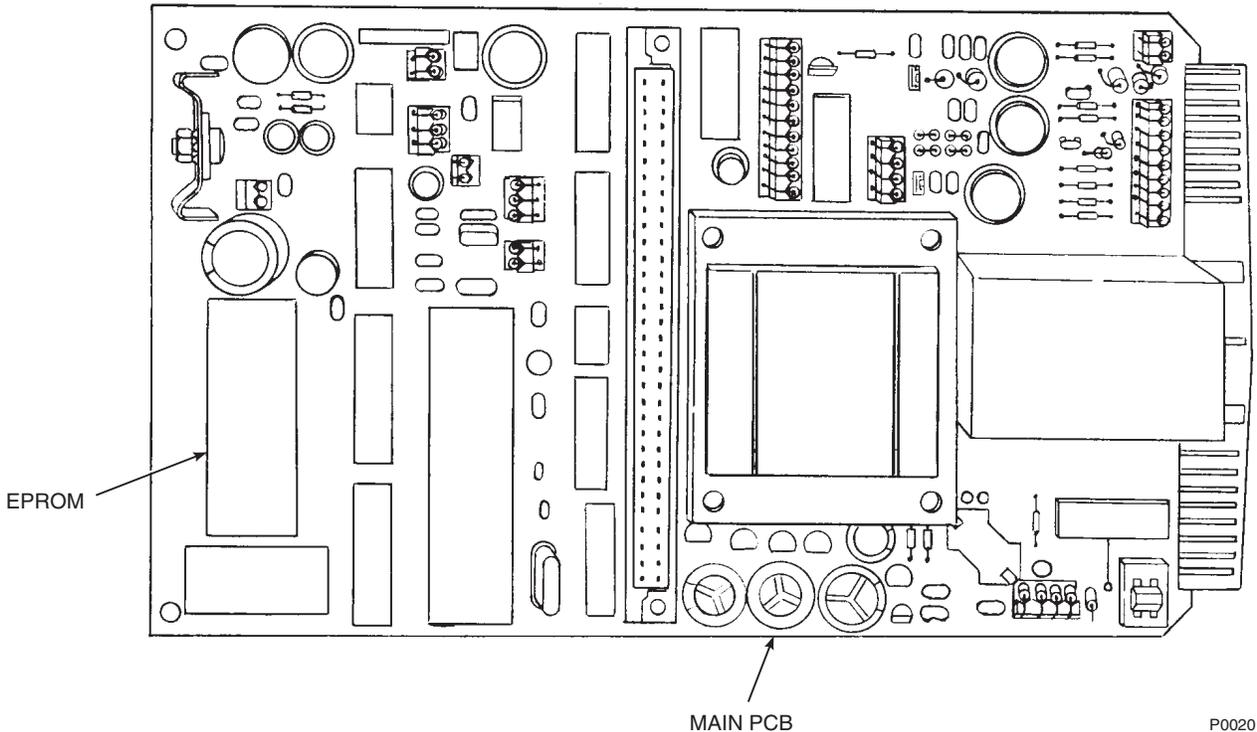
**Figure 2-10. Main PCB (Model 218A) EPROM Replacement**
