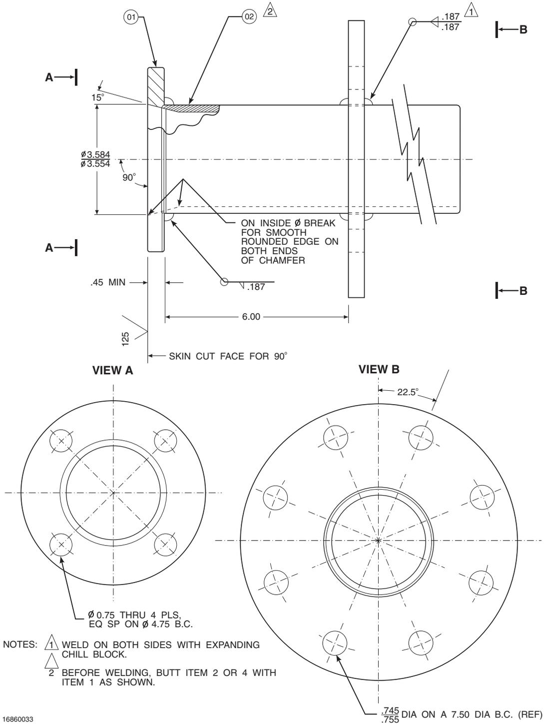
**Figure 1-5. Abrasive Shield Assembly**
