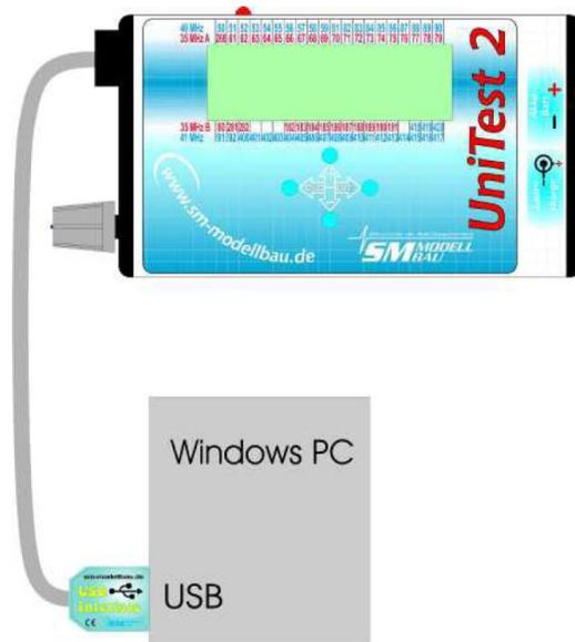
Connect the **USB-Interface** to a free USB port on your PC. Connect the other end to the "**Seriell 1 COM**" connector of the **UniTest 2**.
