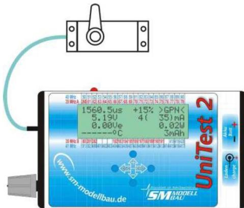
The diagram to the left shows the proper connection of a servo when performing a servo test. The servo can be connected to "**Servo 1**" or "**Servo 2**". You can also connect two servos at the same time. In this case the current consumption displayed by **UniTest 2** is the total current consumption of both servos combined. When connected like this, the servos are powered using **UniTest 2**'s internal battery. This battery has four cells and is comparable to a standard receiver battery.
