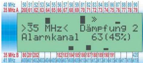
Row 2 shows which frequency band was programmed/detected and the programmed damping amount.
