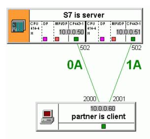
The S7-station has got the IP-addresses 10.0.0.50 und 10.0.0.51 and can be addressed via both connections with the port number 502. The communication partner has got the IP-Address 10.0.0.60 and has to use 2 different port numbers for the two connections: 2000 und 2001
