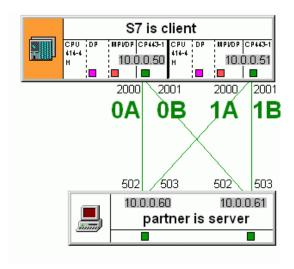
The S7-station has got the IP-addresses 10.0.0.50 and 10.0.0.51. For the access to node A of the communication partner, both CPs, CP0 and CP1, can use port number 2000, because both of them are having different IP-Addresses (connection **0A** and **1A**).
