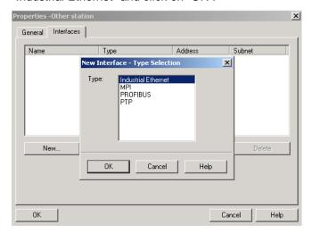
This opens a dialog box "Properties – Ethernet Interface". Enter an IP Address that is in the same subnet as the communication partner's station. The subnet mask should be the same as the one of the partner's station. Select the associated **subnet** that connects the CP interface with the communication partner's interface.
