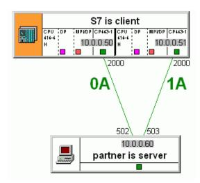
The S7-station has got the IP-addresses 10.0.0.50 and 10.0.0.51 and can use the port number 2000 for both connections. The communication partner has got the IP-Address 10.0.0.60 and must be addressed with 2 different port numbers: 502 and 503.
