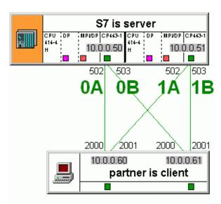
The S7-station has got the IP addresses 10.0.0.50 and 10.0.0.51.for the access from node A of the communication partner. Both CPs, CP0 and CP1, can use port number 502, because both of them are having different IP-addresses (connection **0A** and **1A**).
