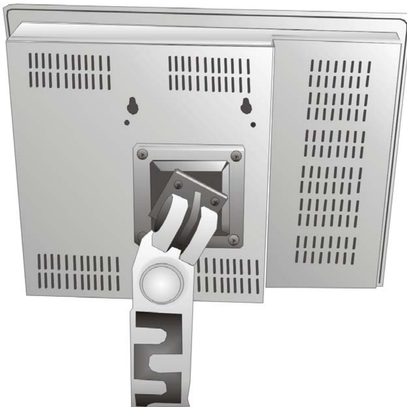
Figure 2-8: Exemplary Swing-arm Installation
