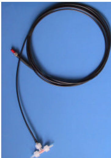
Flow-through cell design connected to a 2 mm POF ( FTC )
