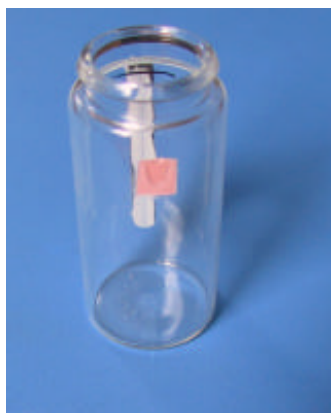
left: Oxygen-sensitive foil glued on the inner surface of a glass vial
