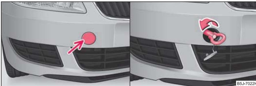
Fig. 161 Front bumper: Cover/installing the towing eye
