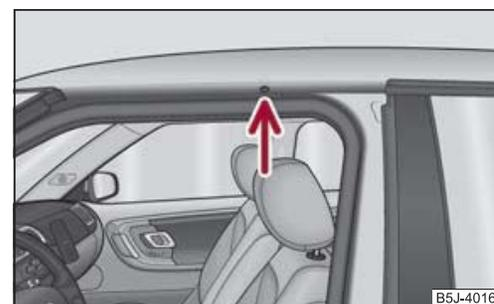
Fig. 73 Attachment points for base roof carrier
