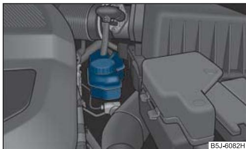
Fig. 144 Engine compartment: Brake fluid reservoir
