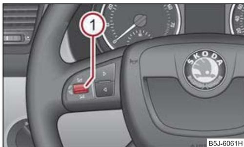
**Fig. 108 Multifunction steering wheel: Mobile phone operation**
