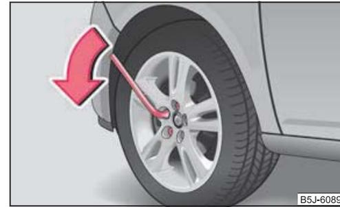
Fig. 155 Changing a wheel: Slackening wheel bolts
