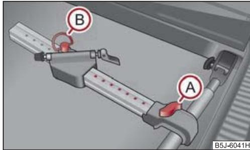
Fig. 70 Install bicycle carrier
