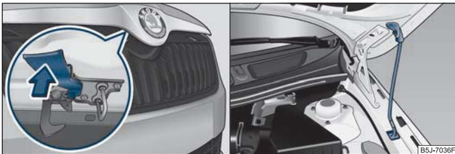
Fig. 140 Radiator grille: Locking lever/securing the bonnet with the bonnet support
