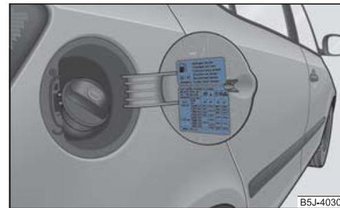
Fig. 148 An opened fuel filler flap with a tyre size and tyre inflation pressure table
