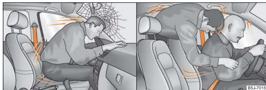
Fig. 111 The driver is catapulted forward if not wearing a belt/The rear seat occupant is catapulted forward if not wearing a belt
