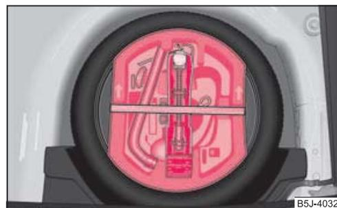
Fig. 151 Luggage compartment: Storage compartment for vehicle tool kit
