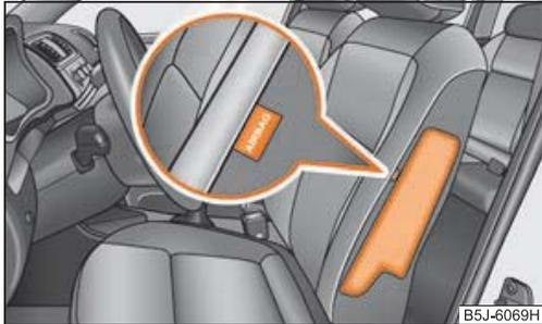
Fig. 118 Driver seat: Installation position of airbag
