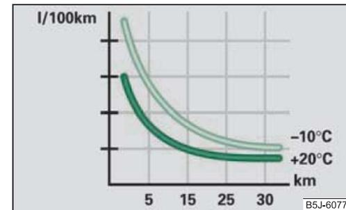
Fig. 136 Fuel consumption in litres/100 km at different temperatures
