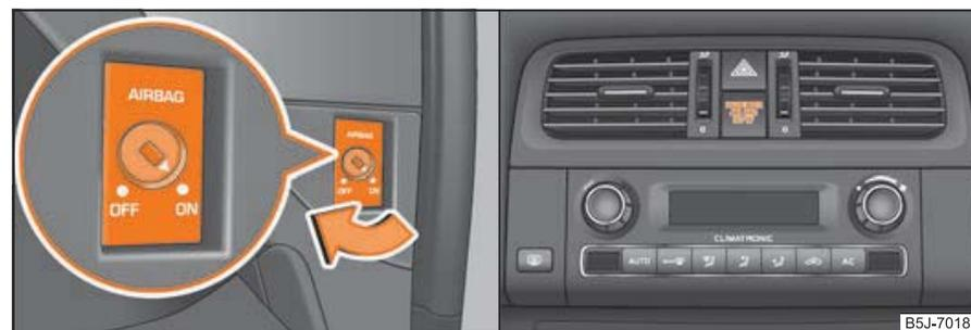
Fig. 122 Switch for the front passenger airbag/indicator light for a switched off front seat passenger airbag
