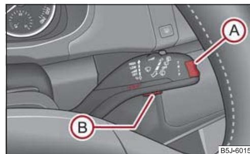
Fig. 19 Multi-functional indicator: Control elements
