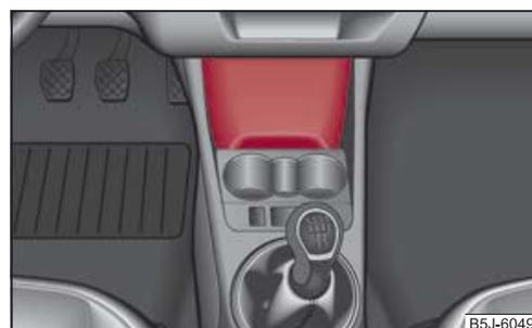
**Fig. 84 Centre console: Storage compartment**
