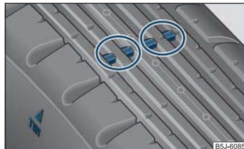
**Fig. 149** Tyre tread with wear indicators
