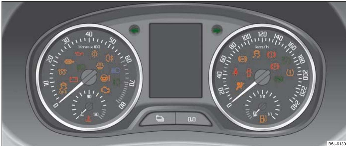
Fig. 21 Instrument cluster with warning lights
