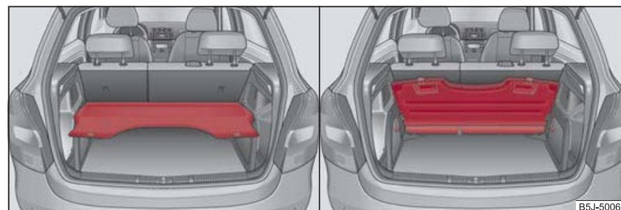
Fig. 61 Luggage compartment cover in the lower position/stowed behind the rear seats
