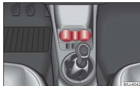
Fig. 74 Front centre console: Cup holder
