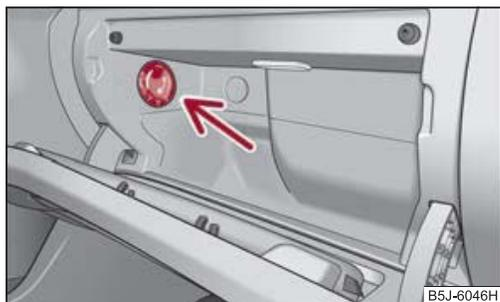
**Fig. 81 Storage compartment: Using cooling system**
