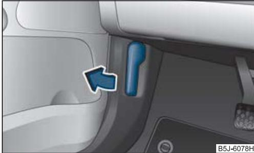
Fig. 139 Release lever engine compartment lid
