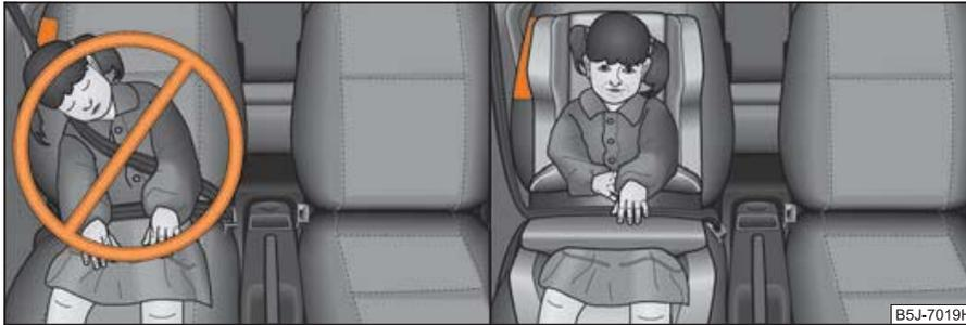
Fig. 124 Unprotected child/Child properly protected by safety seat
