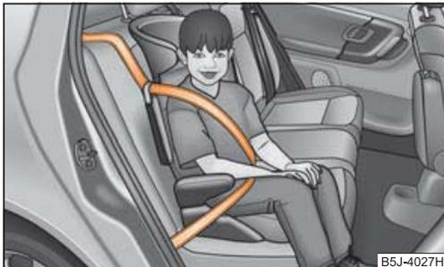
Fig. 127 Child seat in Group 2 installed on the rear seat facing the direction of travel
