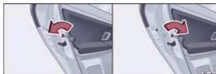
**Fig. 24** Switching child safety lock on: for vehicles without or with central locking system
