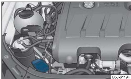
Fig. 147 Engine compartment: Windshield washer fluid reservoir
