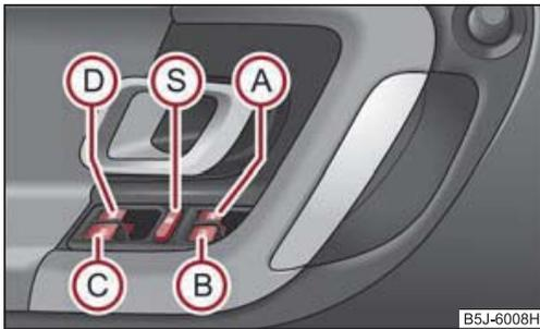
Fig. 10 Buttons on the driver's door
