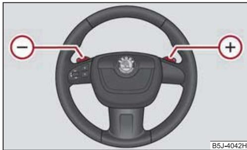
Fig. 103 Multifunction steering wheel: Manual shifting of gears
