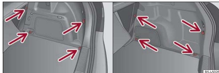
Fig. 57 Luggage compartment: Lashing eyes and fastening elements (Fabia)/(Combi)
