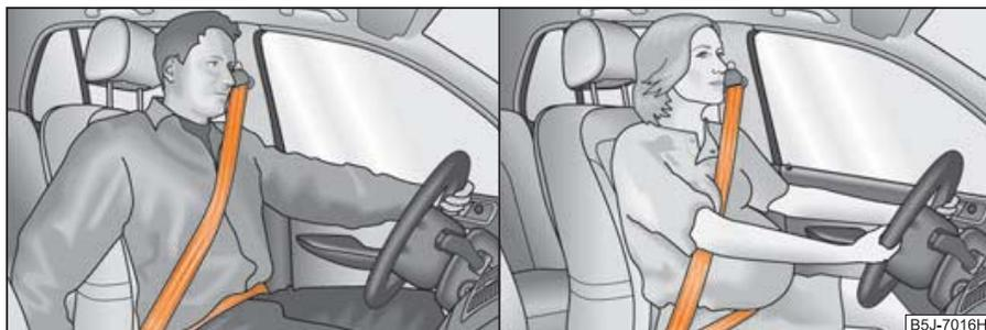
Fig. 112 Routing of belt webbing over the shoulders and the lap belt/Routing of belt webbing for an expectant mother
