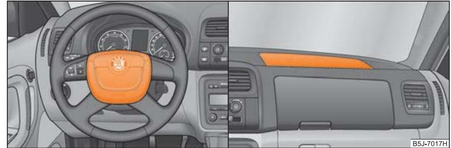
Fig. 115 Driver airbag in the steering wheel/front passenger airbag in the dash panel
