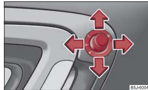
Fig. 6 Inner part of door: Rotary knob
