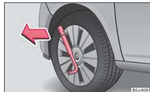
Fig. 153 Removing the full wheel trim ►
