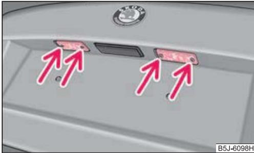
Fig. 176 Remove the licence plate light
