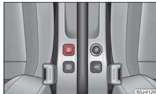
Fig. 100 Centre console: Button for the START-STOP system
