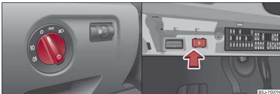
Fig. 35 Dash panel: Light switch/fuse box: Switch for daylight driving lights
