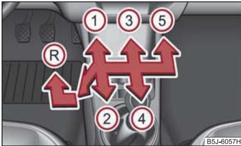
Fig. 96 Shift pattern on models fitted with 5-speed manual gearbox
