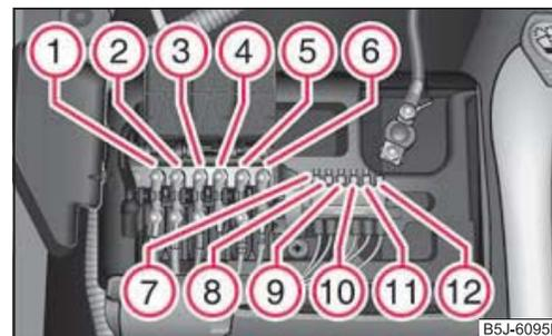
Fig. 168 Schematic representation of fuse assignment at battery
