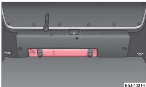
Fig. 150 Placing of the warning triangle
