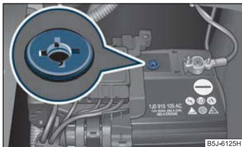
Fig. 146 The battery: Electrolyte level indicator
