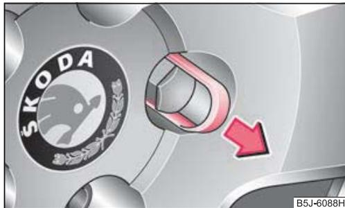
Fig. 154 Changing a wheel: Pull off cap from the wheel bolt
