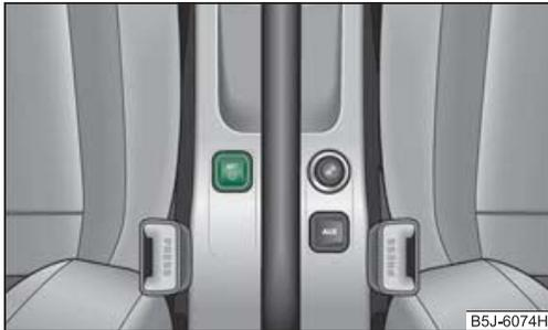
Fig. 132 Button for setting the tyre inflation pressure control value
