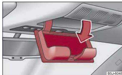
**Fig. 83 Detail of the headliner: Stowage compartment for spectacles**
