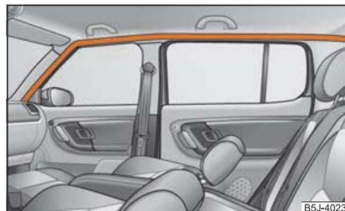
**Fig. 120** Installation position of the head airbags
