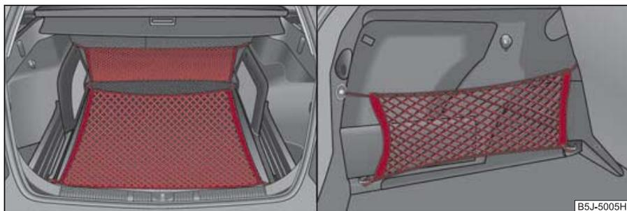
Fig. 58 Fixing net: double horizontal pocket, floor fixing net/double vertical pockets
