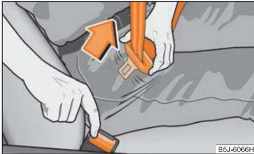
Fig. 114 Releasing lock tongue from belt lock
