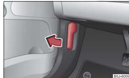
Fig. 12 Release lever engine compartment lid
