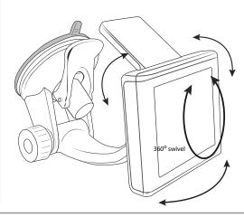
6. To remove, hold the pedestal with one hand and firmly pull Nuvi away from pedestal with your free hand.
