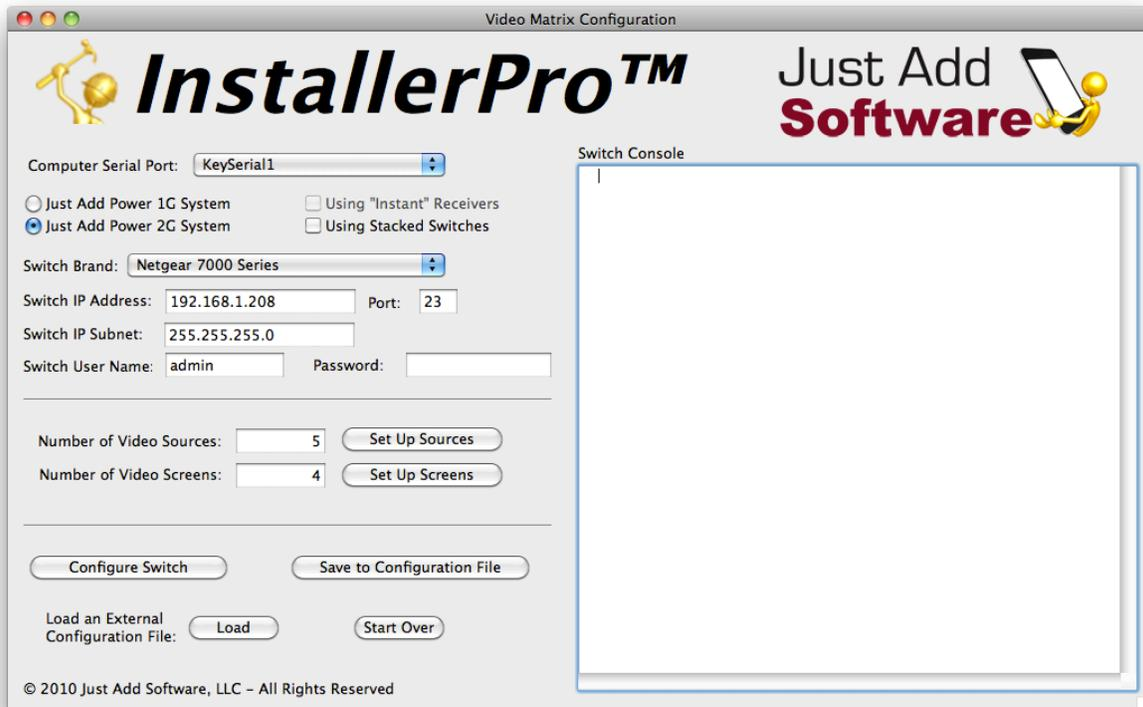
**Select 1G or 2G System:** Select which generation of Just Add Power HD over IP™ product that will be used. The two generations are not compatible and the 2G system requires a gigabit Ethernet switch. The default is 1G.
