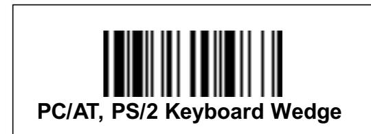
For the keyboard wedge solution, the scanner must work with the existing keyboard concurrently. If you want to link the scanner to a computer keyboard port without a PC/AT or PS/2 keyboard, please select “**Emulate External Keyboard.**” This selection instructs the scanner to perform the power-on handshaking and routine reply between computer and keyboard.
