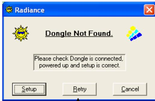
If this screen is displayed, check that the LED on the POD is on, that the PC Comms cable is connected to the PC.
