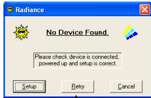
If this screen is displayed, the POD is connected but the Lumina is not communicating. Check that the Lumina is set to cctalk mode (SW7 ON, SW8 OFF)
