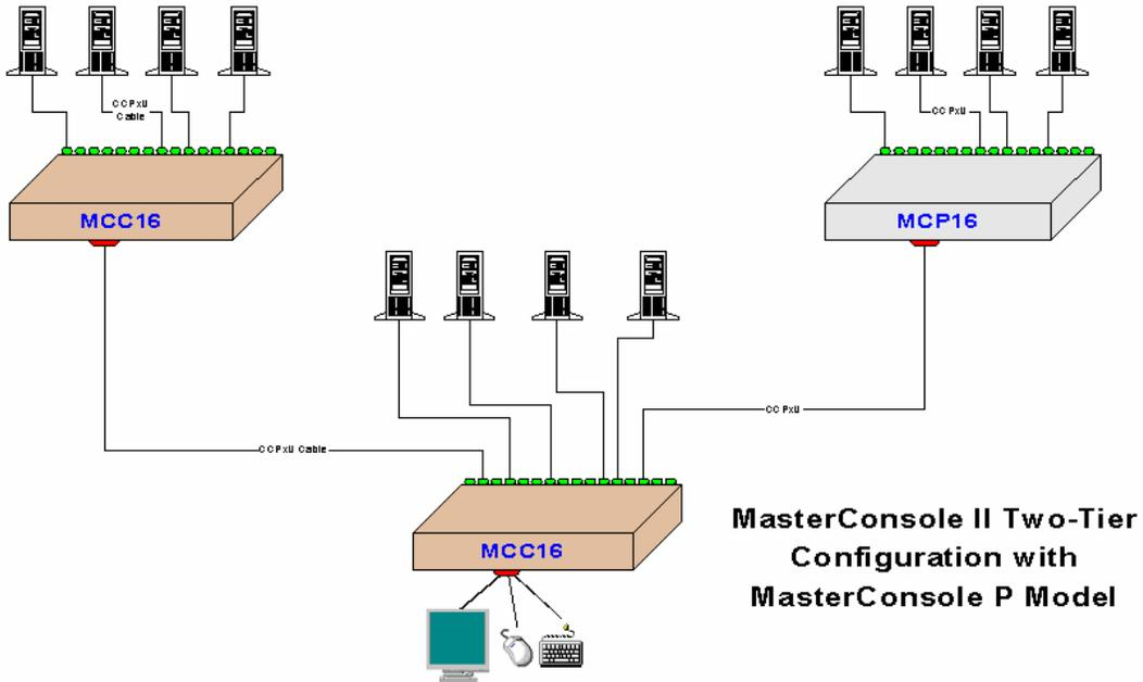
Figure 33 Two-Tier Configuration with MasterConsole P Model
