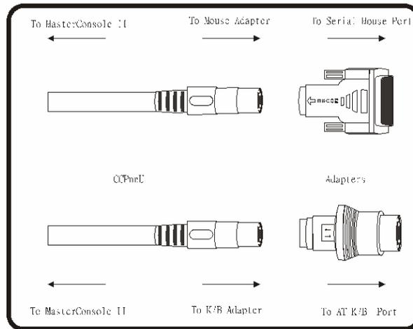
Figure 8 Cable Adapters to Convert PS/2 to AT
