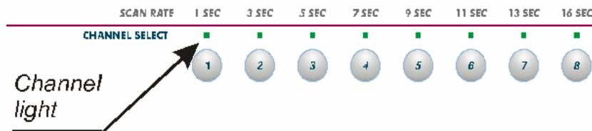
Figure 16 MasterConsole II Front Panel Channel Lights
