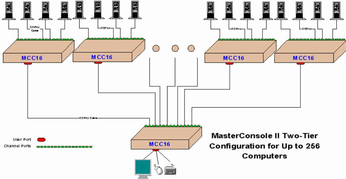
Figure 32 Two-Tier Configuration of up to 256 Computers
