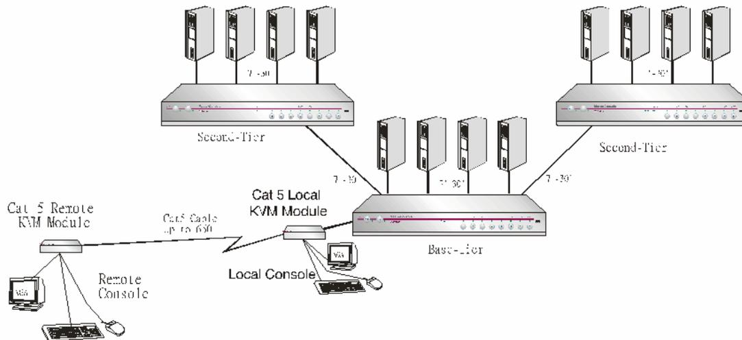
Figure 17 Two-Tier Configuration (with optional Remote Access Kit)
