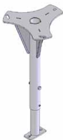
Figure 27. Telescope ceiling bracket, 510 - 850 mm (SWL 300 kg)
