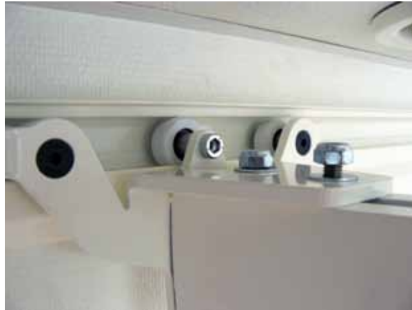
Figure 65. Fitting of traverse rail to telescope trolley and fixed trolley
