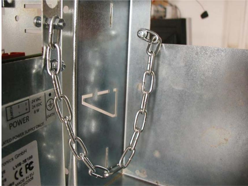
Figure 3: Connecting L-VIS to the wall mount frame.
