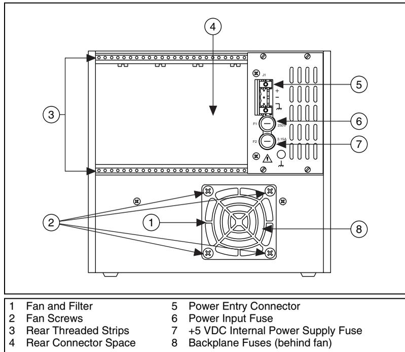
**Figure 2-6.** SCXI-1000DC Rear View Diagram
