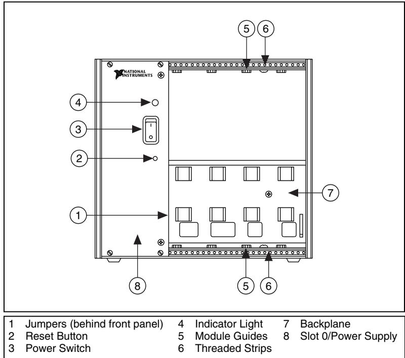
**Figure 2-2.** SCXI-1000DC Front View Diagram
