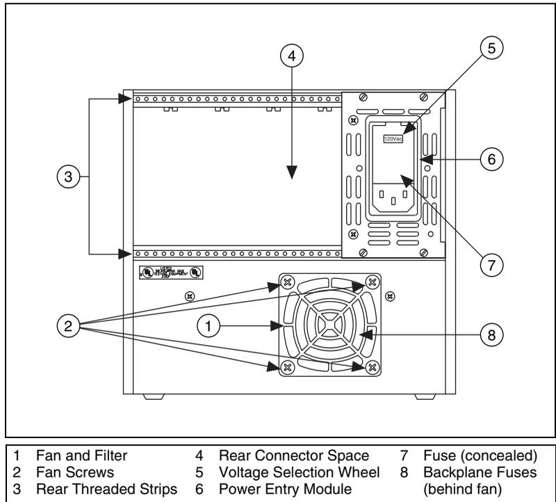
**Figure 2-4.** SCXI-1000 Rear View Diagram
