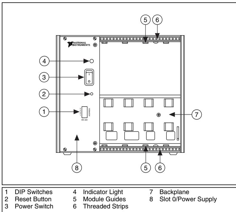
**Figure 2-1.** SCXI-1000 Front View Diagram
