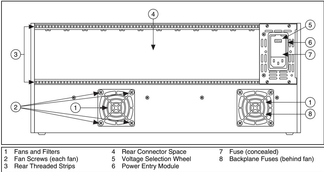
**Figure 2-5.** SCXI-1001 Rear View Diagram
