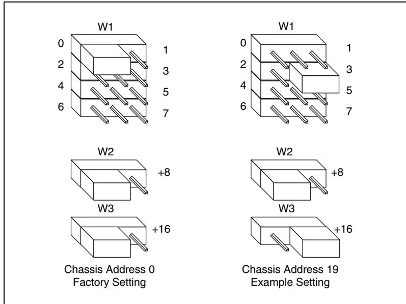
**Figure 2-8.** SCXI-1000DC Chassis Address Jumper Settings
