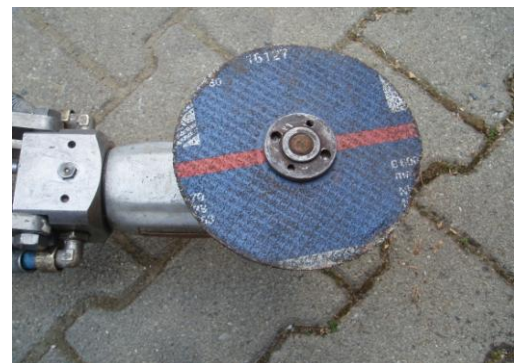
Photo. 2.3.11 (1): milling robot with Steel cutting disk
