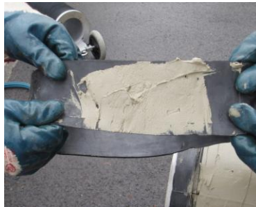
fig. 2.3.7 (2): The coatings flexible qualities
