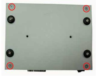
**Step 3** Loosen these screws, and remove the back cover from the system.
