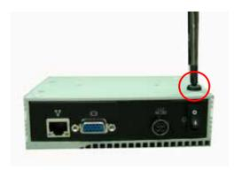
**Step 3** Assembly the bracket to the system, and fasten screws tight.
