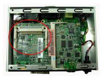
Step 5 Insert the CompactFlash<sup>TM</sup> card into the socket until it is firmly seated.
