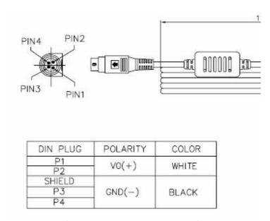
(Figure - Power Adapter Pin Assignment)
