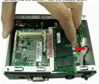
**Step 6** The memory module is locked by two latches on the sides.
