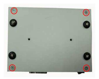
**Step 3** Loosen these screws, and remove the back cover from the system.
