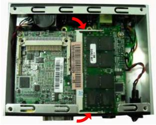
NOTE While uninstalling the Memory Module, you need to stretch these two latches aside, and then take the module off the socket.
