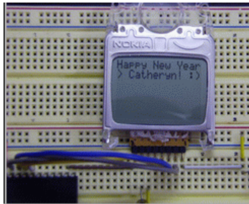
Figure 2.5: Nokia 3310 PCD8544 Based Graphical LCD Demo
