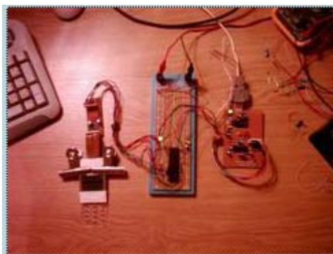
Figure 2.4: Nokia 3310 LCD Driver using a PIC
