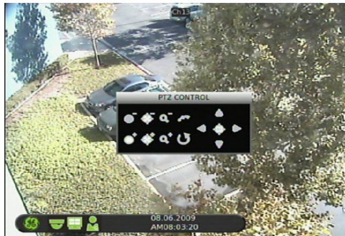
Figure 12: PTZ control interface
