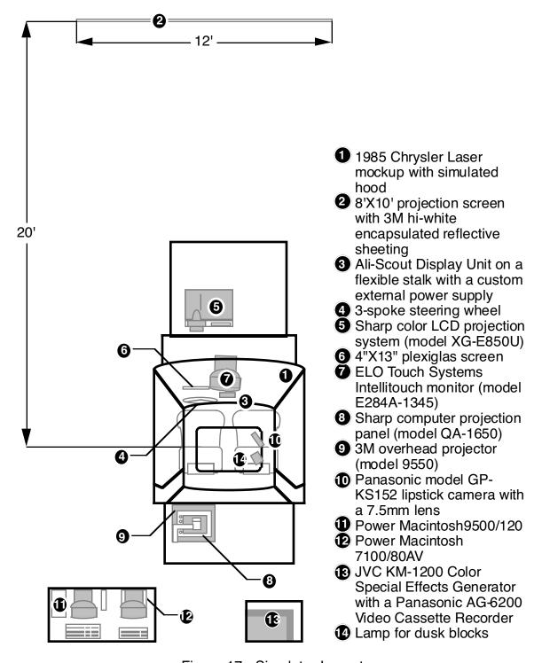
Figure 17. Simulator Layout
