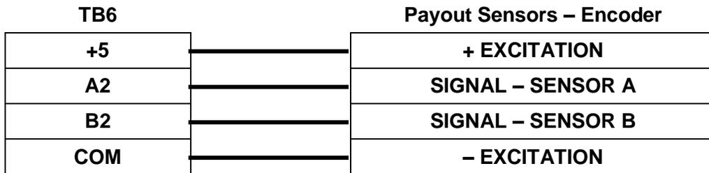
Figure 4.15 – Rotational Sensor Hookup – TTL Encoder, Counter 2
