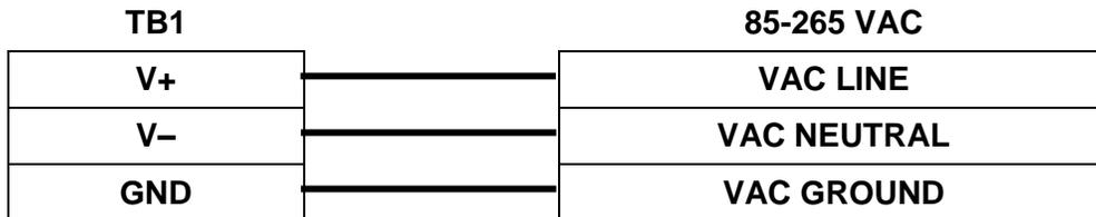
Figure 4.28 – Remote Display Power Hookup – AC Power
