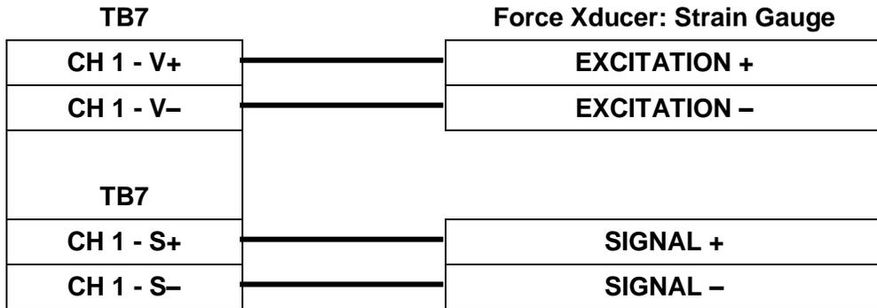
Note: 4-wire strain gauge default range is 20 mV full scale.
