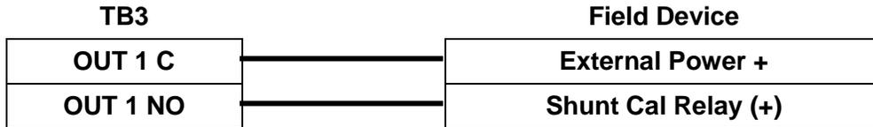
Note: Shunt Cal relay power must be referenced to external power common.
