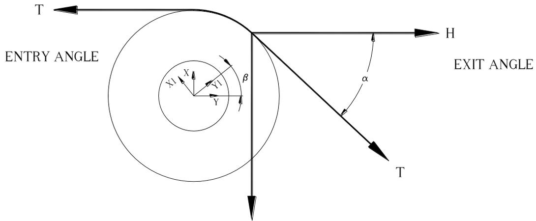
In an actual installation the load pin may not be aligned such that the y-axis of the load pin is exactly parallel to the winch line. The LCI-90 has the ability to correct for this orientation error. In the example above the load pin is oriented along X1 and Y1 axis. The idealized condition discussed in the previous section had the load pin oriented along the X and Y axis. The angle  $\beta$  is the Sensor Angle specified in the 2.0 Calibration menu.
