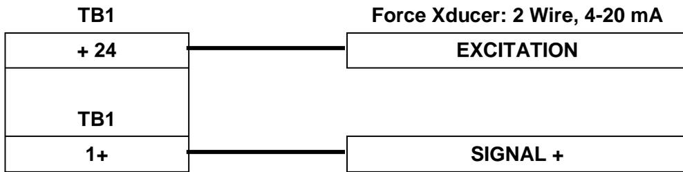
Figure 4.7 – Tension Hookup – 2 Wire 4-20 mA Signal
