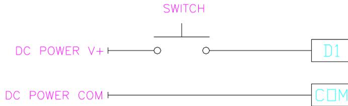
Figure 6.1 – Wiring Digital Input 1 External Power
