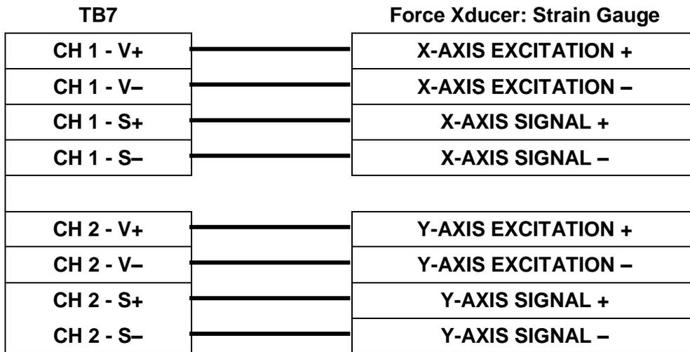
Note: Each 4-wire strain gauge module must be inserted in correct position.
