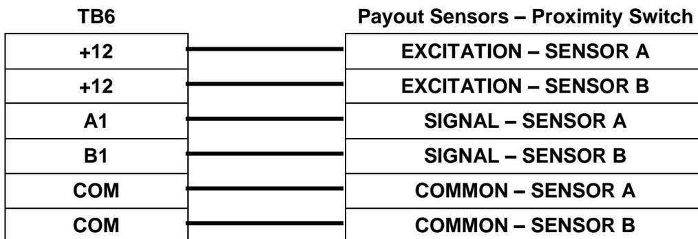
Figure 4.13 – Rotational Sensor Hookup – 12V NPN/PNP switches, Counter 1
