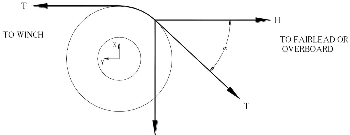
Note: This is the idealized condition where the  $Y$ -axis is parallel to the line going to the winch. This is a fixed relationship, but as the equations below show,  $\alpha$  can vary without changing the calculated Tension.
