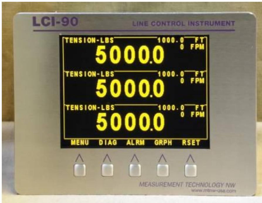
Figure 5.8 – LCI-90i Triple Winch Mode
