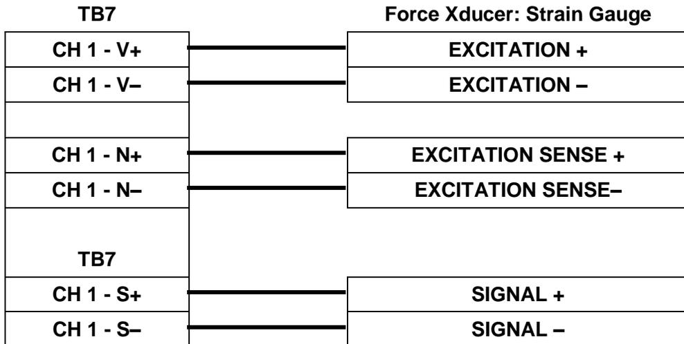
Note: 4-wire strain gauge default range is 20 mV full scale.
