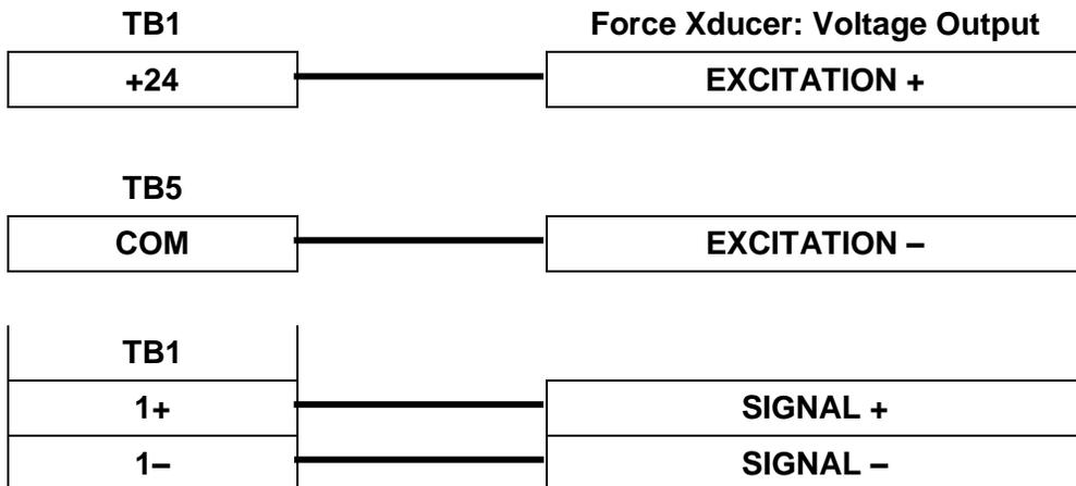
Figure 4.8 – Tension Hookup – 4 Wire DC Voltage Input
