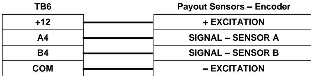
Figure 4.14 – Rotational Sensor Hookup – Hall Effect Sensor, Counter 4
