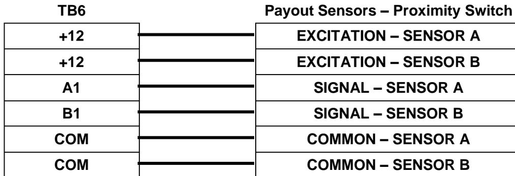
Figure 2.3 – Payout Hookup – 2 Channel 12VDC Proximity Switch
