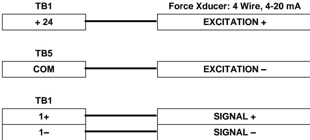
Figure 4.6 – Tension Hookup – 4 Wire 4-20 mA Signal
