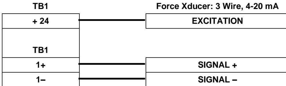
Figure 4.5 – Tension Hookup – 3 Wire 4-20 mA Signal
