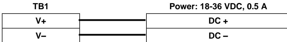
Figure 4.27 – Remote Display Power Hookup – DC Power
