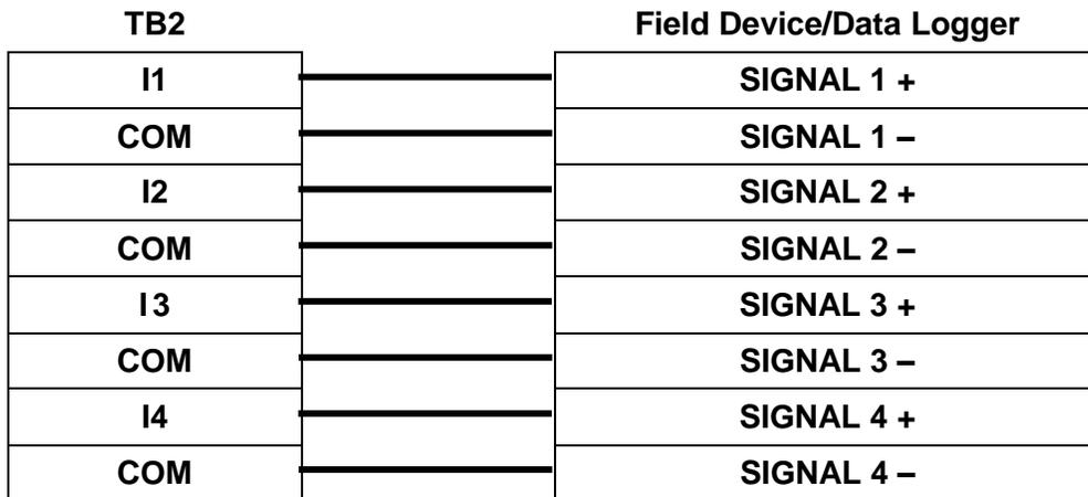
Figure 4.20 – 4-20 mA Current Output Hookup – 2 Channels
