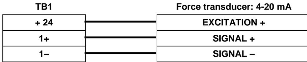
Figure 2.2 – Tension Hookup – 3 Wire 4-20 mA Signal
