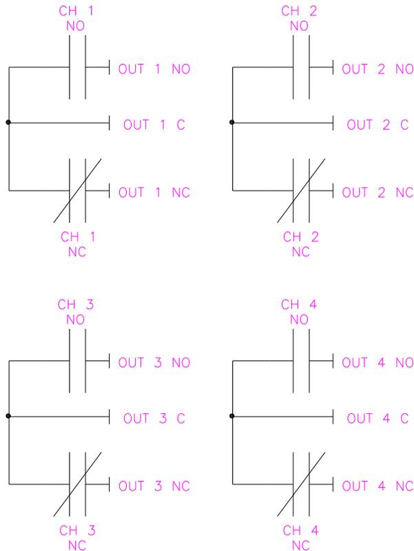
Figure 4.17 – Alarm Output Hookup – 4 Channels - Ladder Logic
