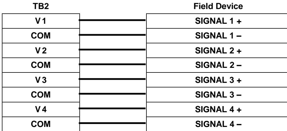
Figure 4.19 – Voltage Output Hookup – 4 Channels
