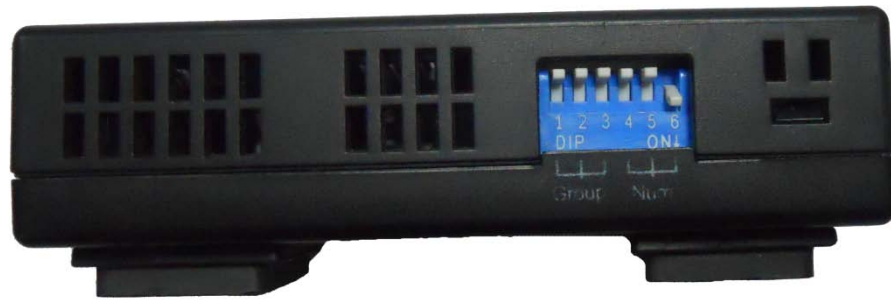
Figure 8-7 DIP switch of temperature sensor
