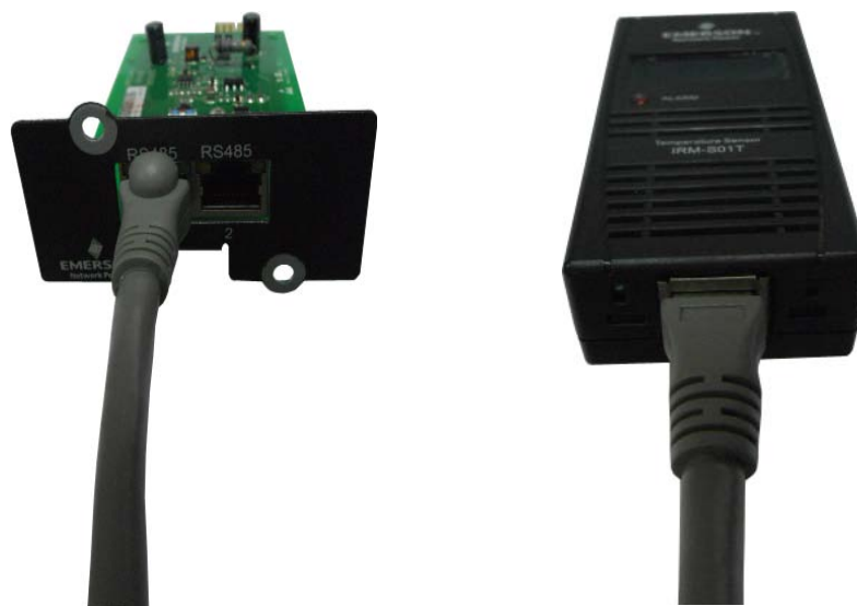
Figure 8-6 Connection between UF-RS485 card and battery temperature sensor
