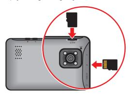
To remove a card, gently push the top edge of the card inwards to release it, and pull it out of the slot. Inserting the card in the reverse direction may cause damage.
