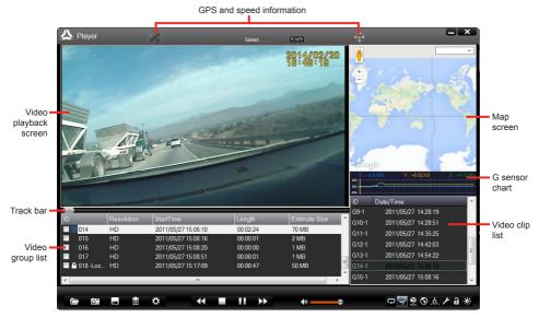
**Note:** G sensor chart displays data in 3-axis waveform about the car's shift forward/backward (X), to the right/left (Y) and upward/downward (Z).
