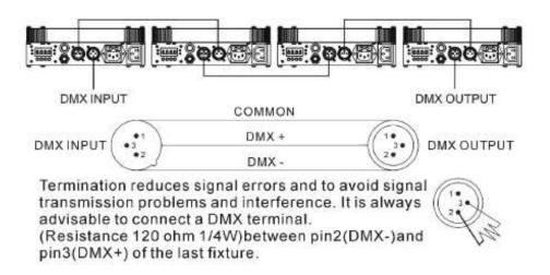
• If you are using a controller with 5-pin DMX output, use a 5-pin to 3-pin adapter cable.
